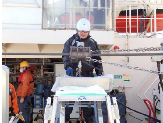
(b) Grease apply during pay out
