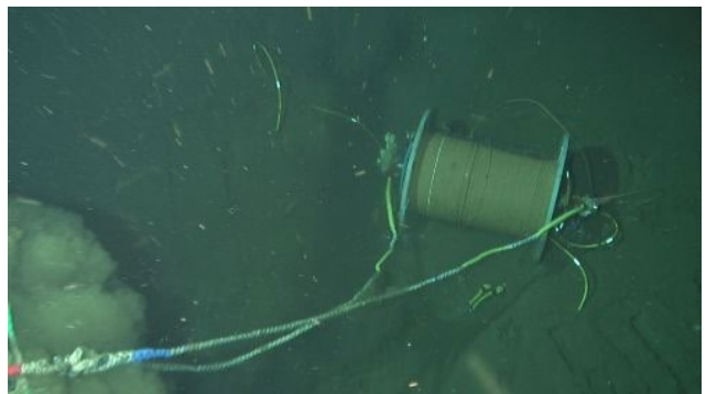
Photo 4.5-10 Connect a retrieval rope to the Extension Cable Bobbin No.42.
