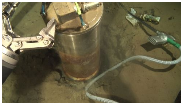
Photo 4.4-3 Lifting up the Ground Motion Sensing System (JB#29).
