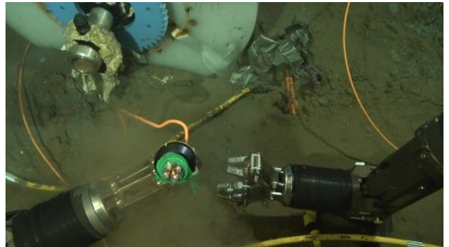
Photo 4.5-6 The extension cable (orange cable) through into the cable catcher.
