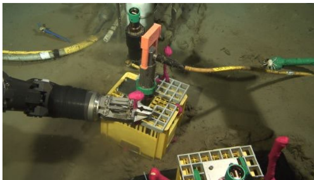
Photo 4.2-3 Connect to the loopback connector for investigation from the Yokohama Backup Site.
