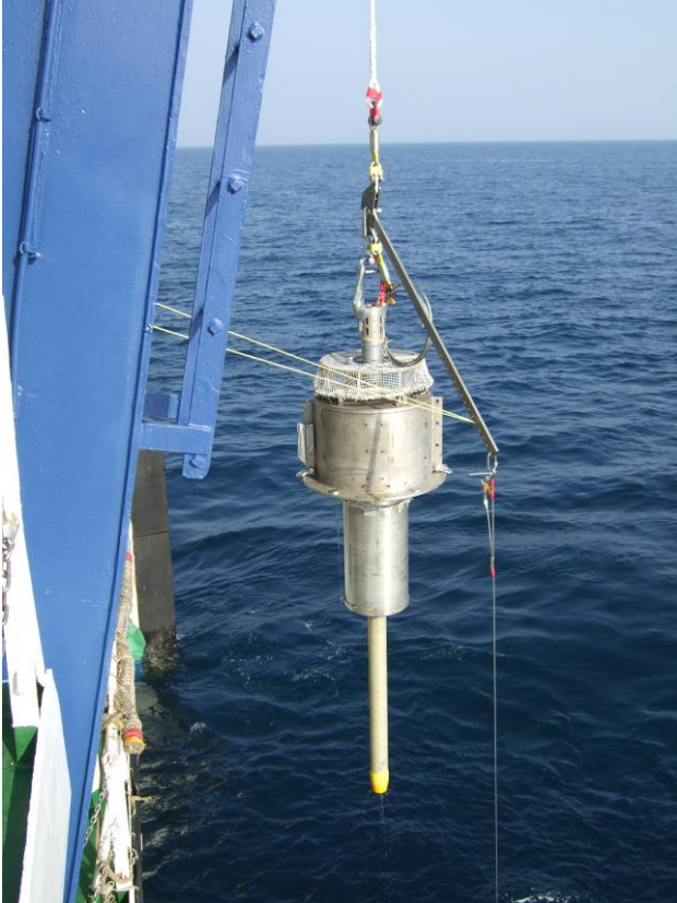
Benchmark installation from the vessel.
