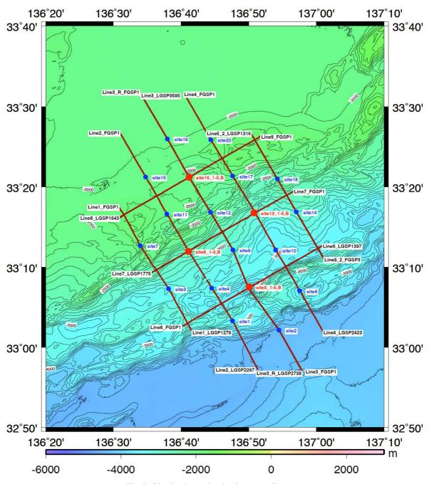
Fig.2. Single channel seismic suvey lines.
