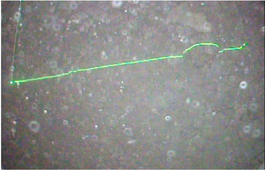
Fig. 6 Example of laser profiling during this cruise with lights on in turbid water
