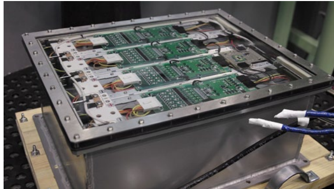
Figure 3.2.2: Lithium-ion battery unit.
