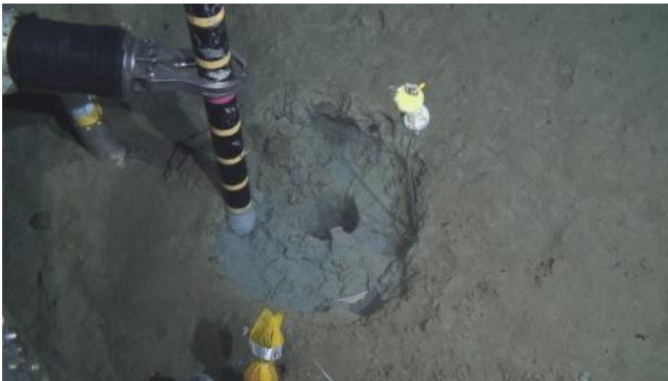
Photo 18 Burial hole conditioning operation of the observatory C-9 candidate
