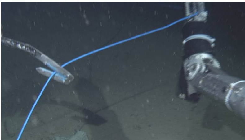
Fig. 3.19 Extension cable released from the cable bobbin
