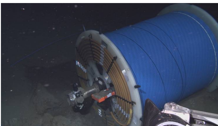
Fig. 3.12 Cable bobbin deployed on the way
