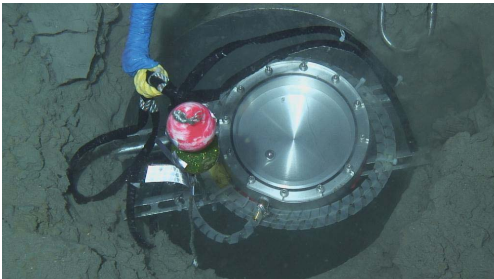
Fig.3.18 Check the horizontal error of the casing
