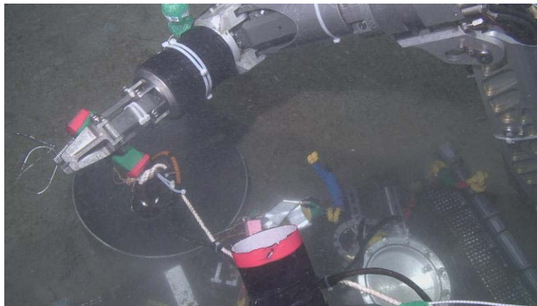
Fig. 3.3 Check the inside of casing by the auxiliary camera
