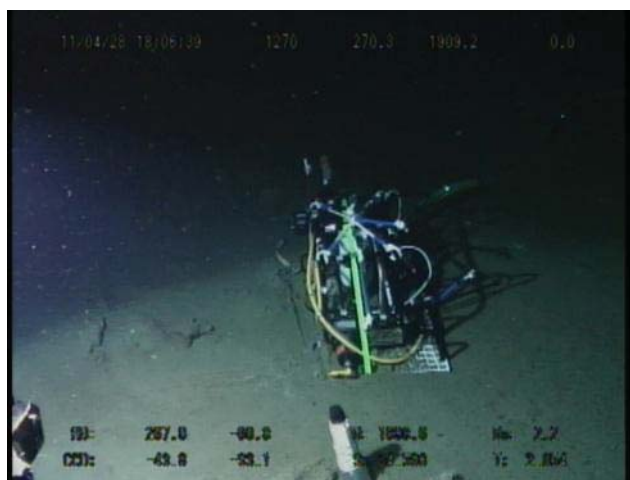
Fig.3.16 Sensor package and miniature transponder
