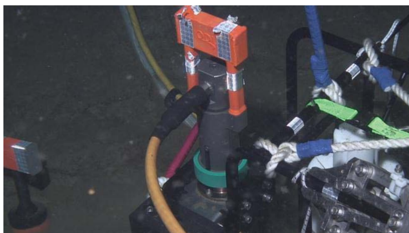
Fig3.34 The other end of extension cable was connected to the sensor package
