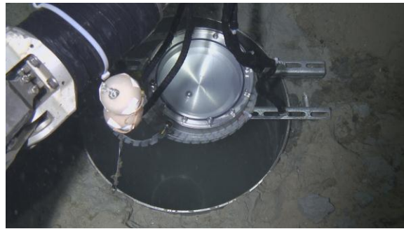
Fig. 3.2 Check of the inclination angle by the level-meter
