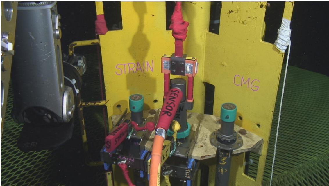
Figure.9 Photos of ROV I/F connection to strainmeter (top) and tilt combo (bottom).
