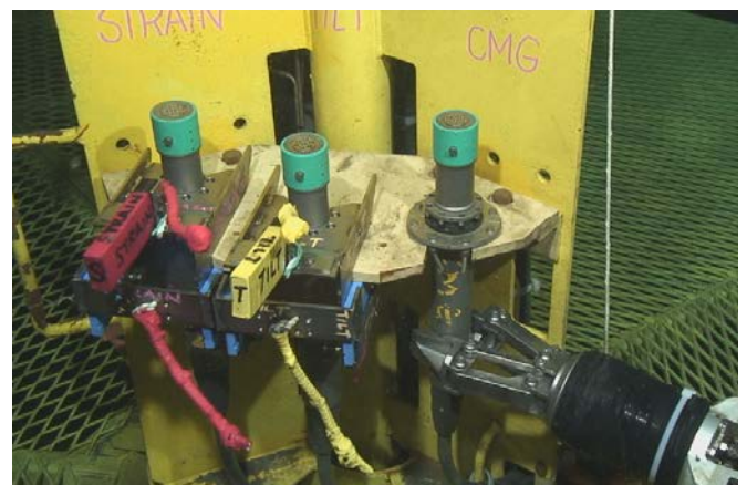
Figure 7 The attachment of the connector protector tools for the LTBMS sensors.
