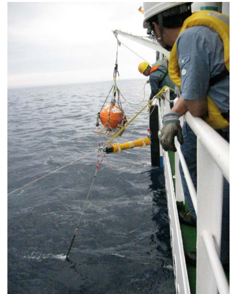
5) Loosen the rope fastening the anchors to the cleat and move their own weight to the instruments.
