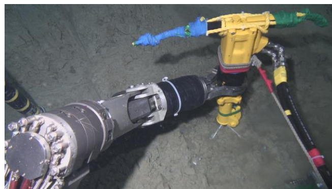
Fig. 3.3 Performance check of the new casing installation device
