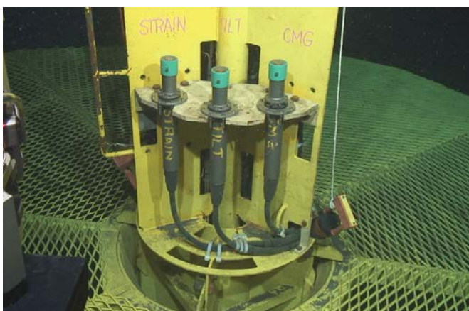
Figure 7 The attachment of the connector protector tools for the LTBMS sensors.
