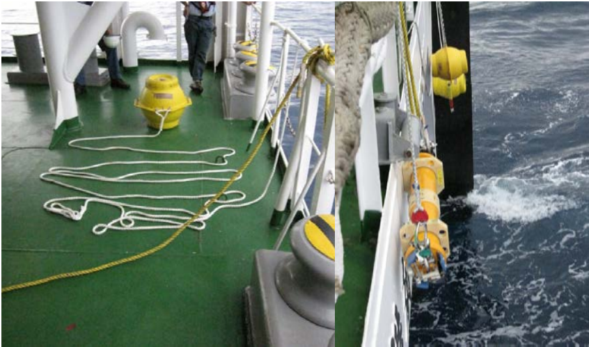
1) Tighten the mooring system from the top buoy to the transponder to the hand rail with the ropes.
