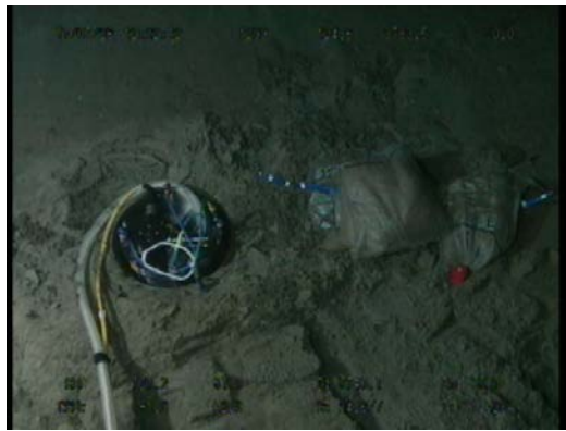
Fig. 3.4 The seismometer package and sand bags
