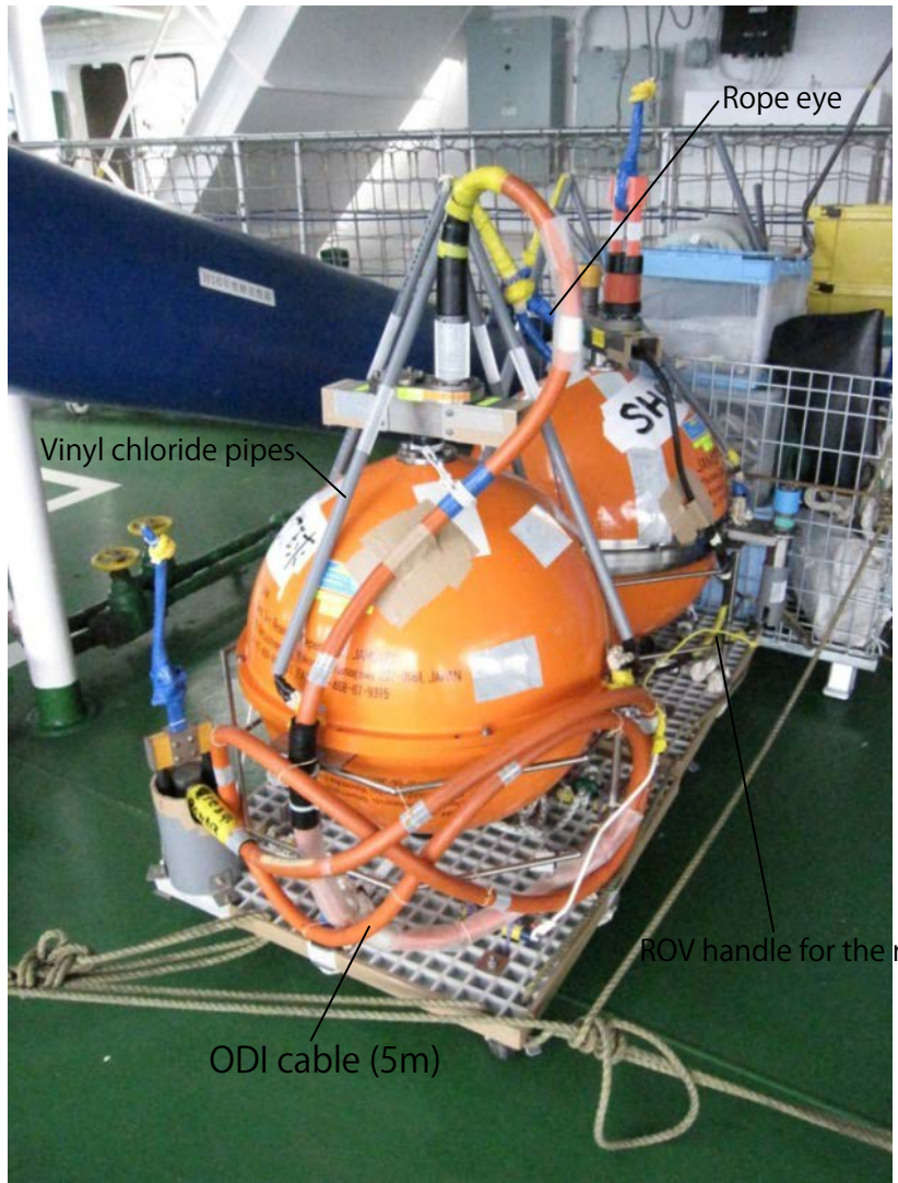
Battery instrument for long term monitoring
