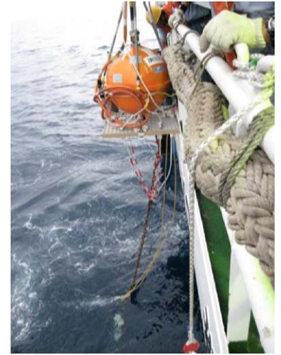
4) Pick up the instruments (SAM, Repeater and Battery) to the outside through the transponder davit with Sea catcher for release.
