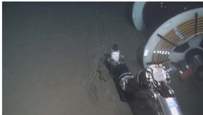
Fig. 3.9 The miniature transponder; ID: 11
