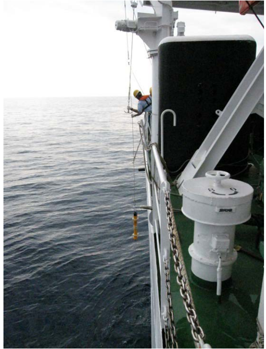
3) Recover the transponder with releaser.
