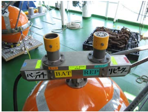
UMC connectors Left: Male connector for the battery Right: Female connector for the Repeater
