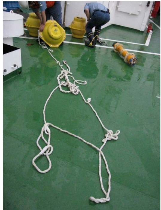
4) Recovered the mooring system from the top buoy to the transponder.
