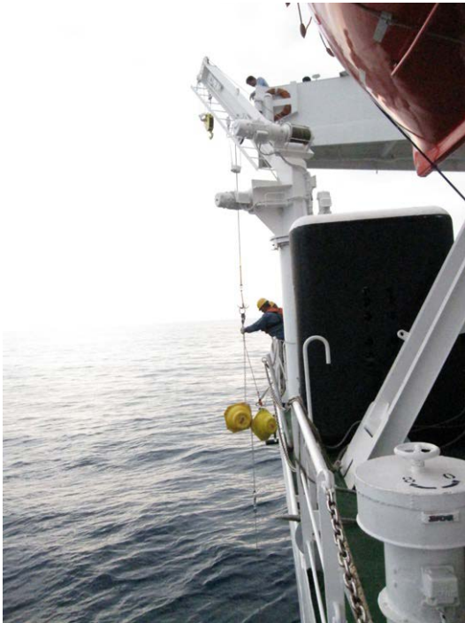
2) Picking up the buoys using the crane on the working deck at the port side.
