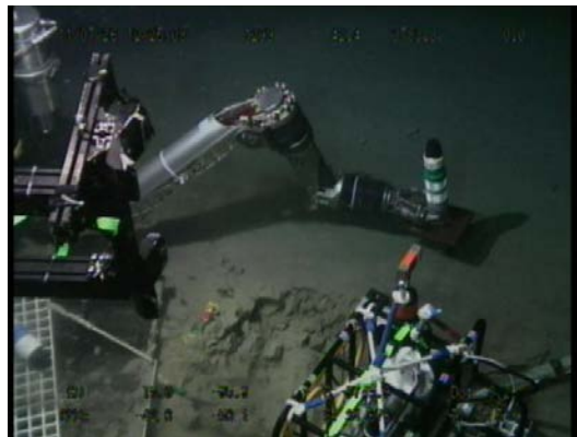
Fig. 3.5 The pressure-gauge sensor package and the miniature transponder
