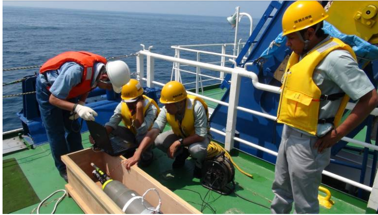
Fig. 9: Final checks of the prototype of deep floats just before deployment (at the second deployment on 12 th August).
