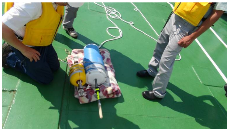
Fig. 3: The surface GPS buoy used in the tests.
