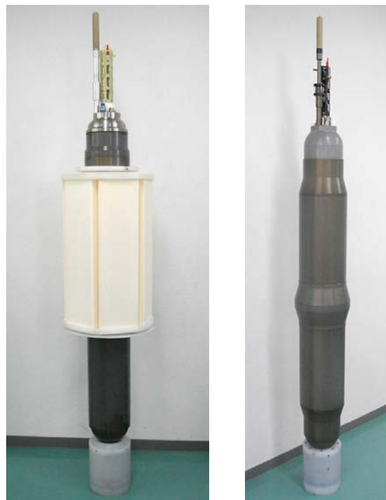
Fig. 1: (a) The demonstrator of the buoyancy engine for the VM shuttles (left) and (b) a prototype of deep profiling floats (right).
