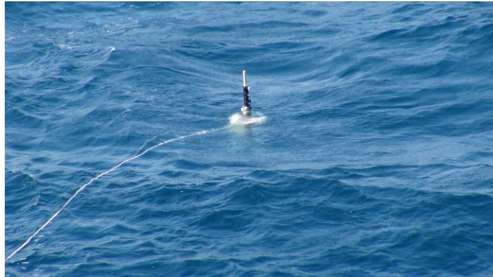
Fig. 6: The VM demonstrator in the test (1) and (2). The demonstrator transmitted its positions fixed by GPS to land-stations via Iridium satellites every 10 minutes successfully while it drifted on the sea surface for about an hour.
