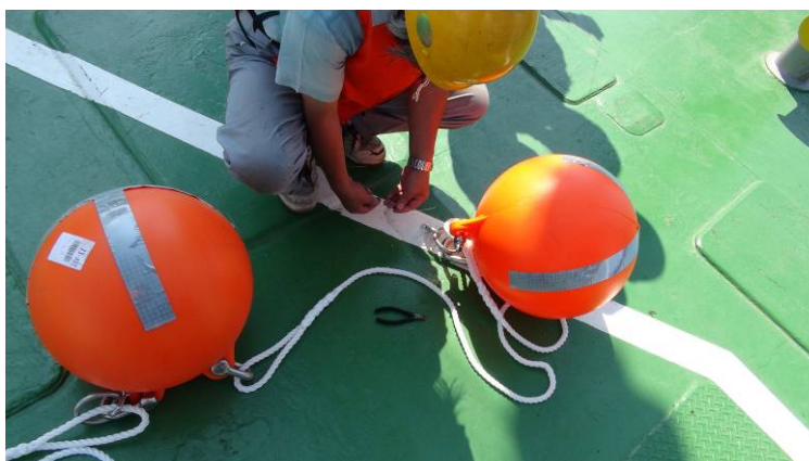
Fig. 4: Surface drifting buoys just before deployed.
