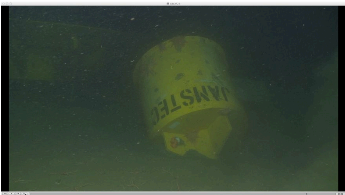
Figure 15. A dropped corrosion cap.
