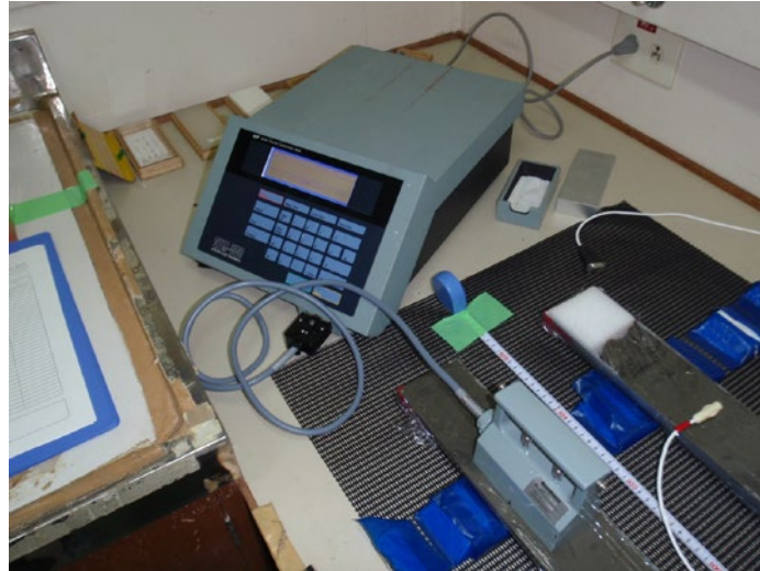
Figure 3.4-7. Thermal conductivity measurement with QTM-500.
