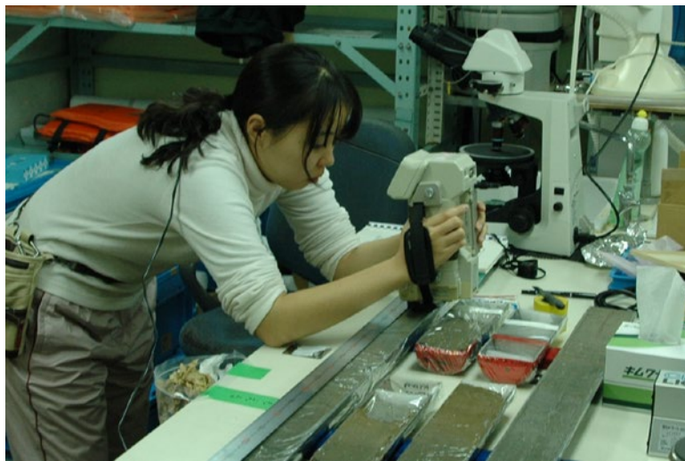
Figure 3.4-9. Sediment color reflectance measurement on the sample KY12-14 HFPC01 with CM-2022 photospectrometer.
