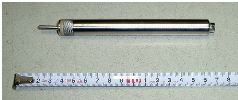
Figure 3.4-2. ANTARES Miniaturized Temperature Data Logger (MTL).
