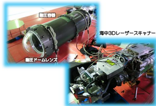
Figure 2-2 Underwater laser-scan system.
