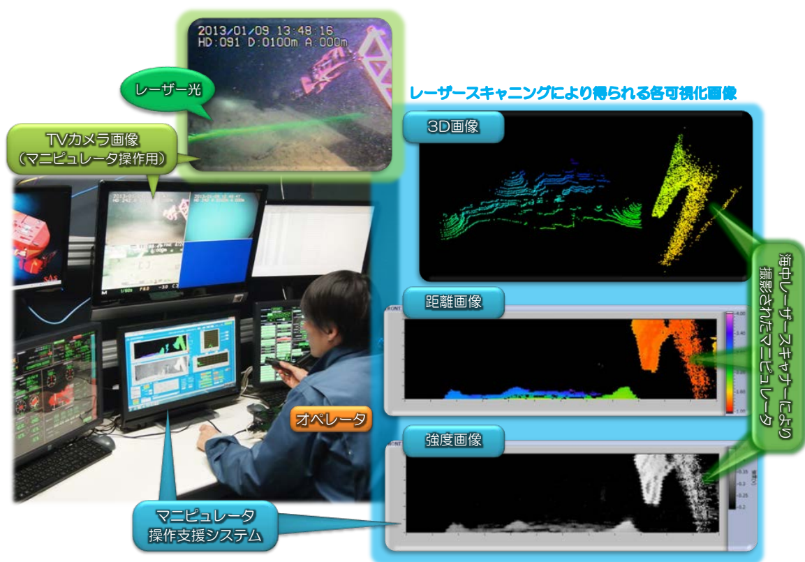
Figure 2-4 A scene of the manipulator operation using 3D image of the circumference environment.
