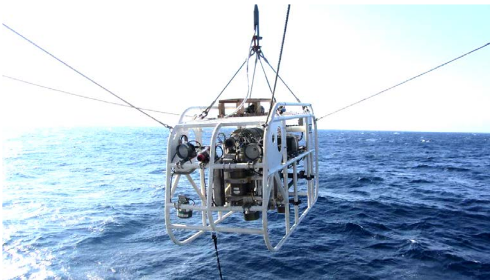
Fig.4.3 The underwater unit of 6,000m-class Deep Tow camera system
