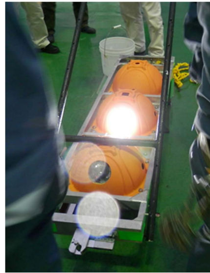
LED light is lit for Unit No.3 was operating continuously.
