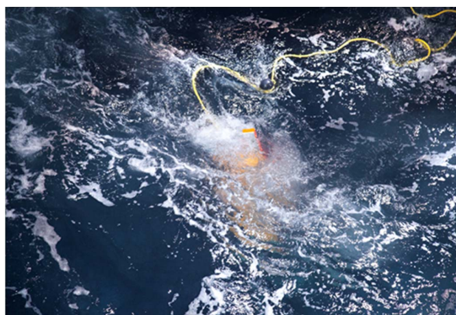
Unit No. 2 which floated at sea. The rope of the buoy was developed normally.
