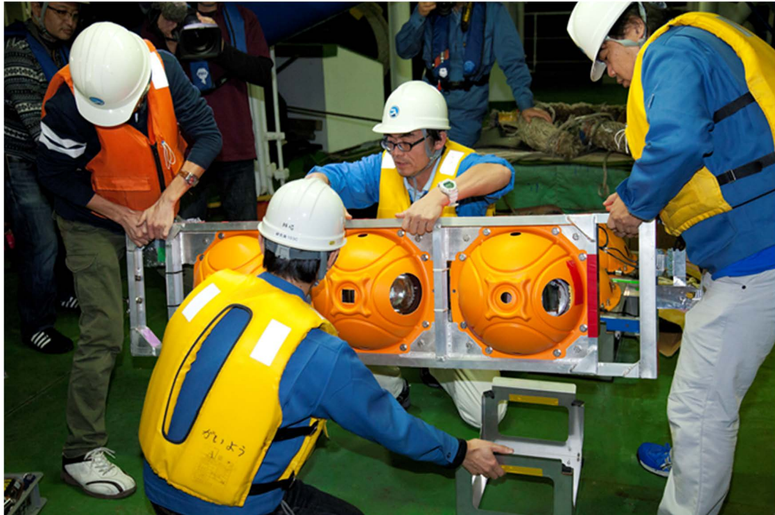
Under maintenance of the Unit No. 2. A lighting sphere (center) and a camera sphere (right)
