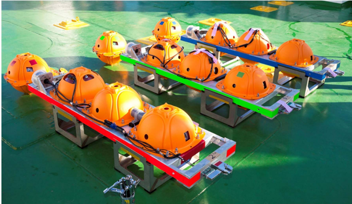
Eddoko - 1 Free-fall camera system such as unit No.2 (red), unit No.3 (green), and unit No.4 (blue) on the deck of R/V Kaiyo.
