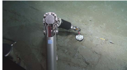
Fig.4.15.4 Leveling of the seismometer
