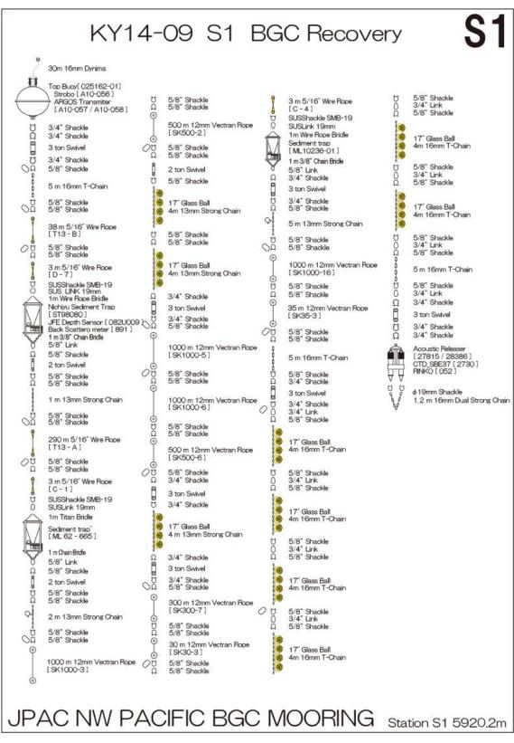
Figure A1. Recovery BGC Mooring Figure at S-1
