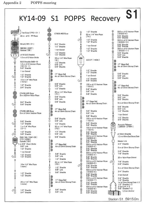
Figure A3. Detailed design of the POPPS mooring recovered at station S1 in KY14-09.
