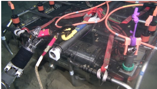
(c) Connecting the hook for recovery to Node 2D
