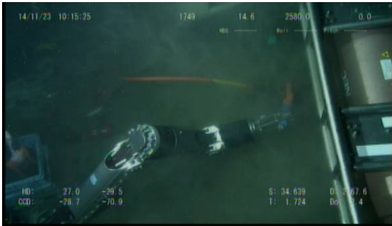
(a) Pulling out the UMC from TU-2D.
