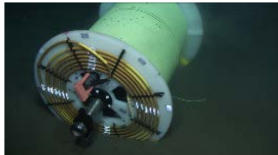
(d) Cable bobbin was putted on near the sensor
