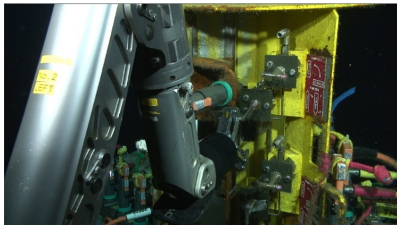
(b) Valve operations of the pressure sensors in the C0002 borehole
