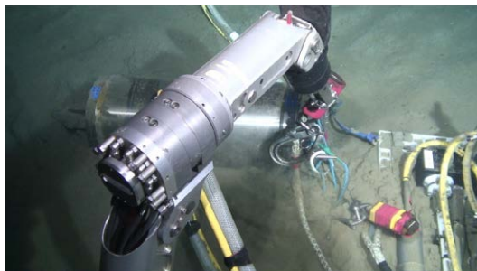
(c) Hooking the rope for recovery
