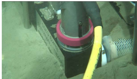
(c) Battery package was connected to the pressure sensor package.
