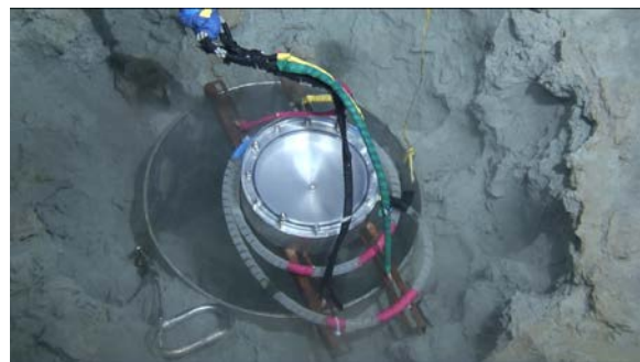
(b) Measuring the tilting angle
