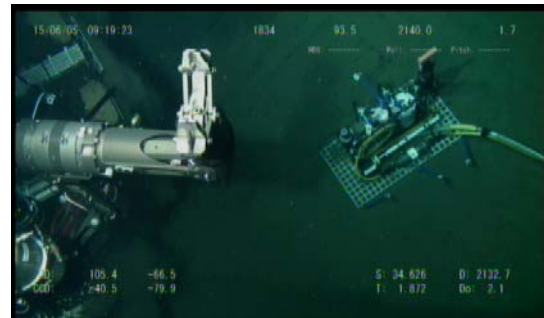
(b) Pressure sensor package
