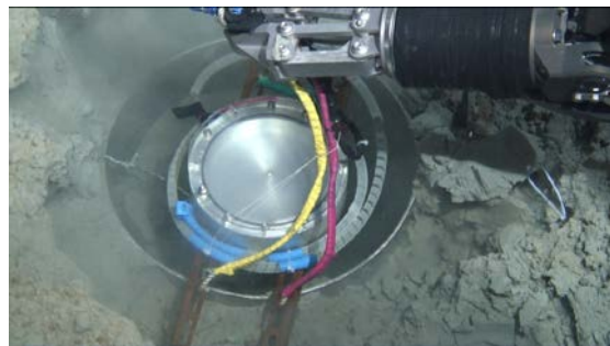
(b) Measuring the tilting angle
