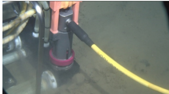
(d) The battery package and the sensor was connected
