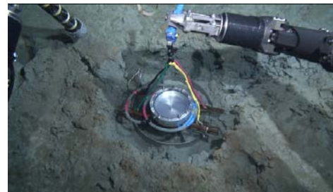
(b) Measuring the tilting angle
