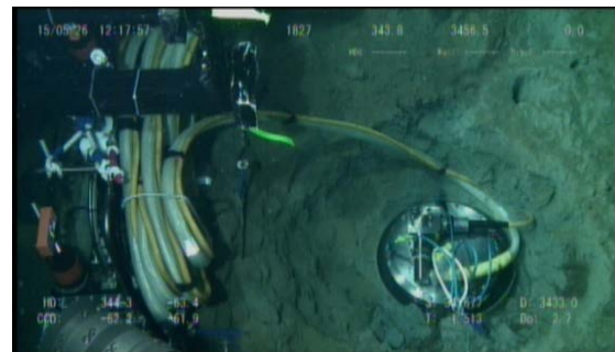
(b) Installation of the seismometer
