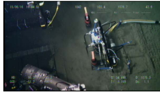
(b) Pressure sensor package
