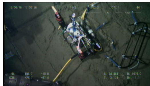
(d) Battery package was connected to the pressure sensor package
