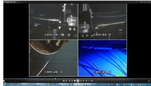
(b) The cable on the cable bobbin got tangled
