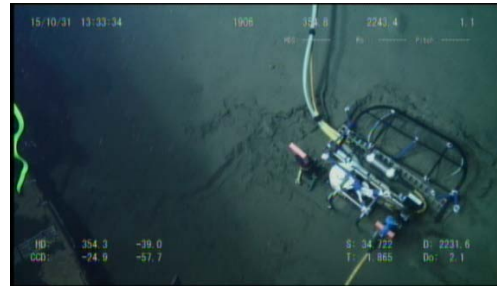
(d) Pressure sensor package connected with battery equipment
