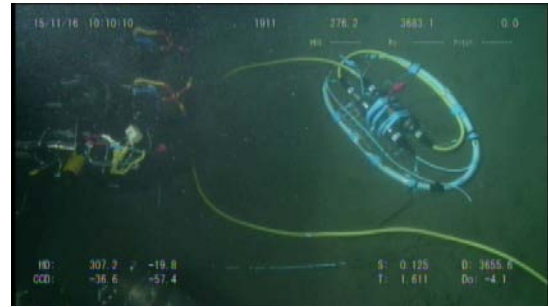
(b) Placing the junction box on the seafloor
