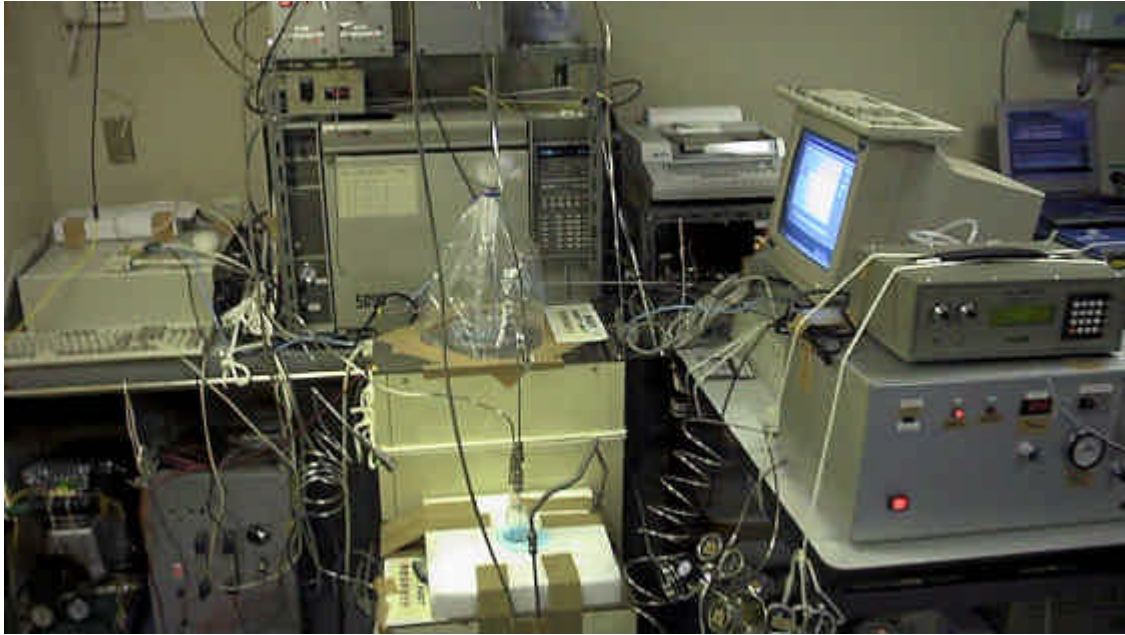
Figure 1. Measurement system for atmospheric O 2 / N 2 ratio on board Mirai. The system includes an automated gas chromatograph, sample injector, cryogenic traps, and NDIR for atmospheric CO 2 measurement.
