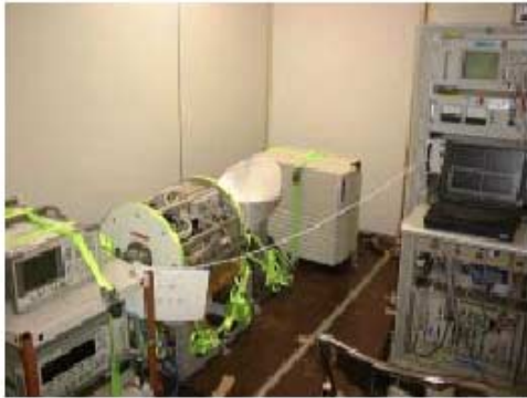
Fig. 1: 95GHz cloud profiling radar for shipborne measurement.
