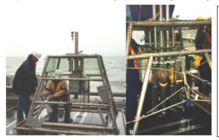
Figure 6. A. Multicorer being prepared by installing 4 Plexiglas tubes on each side of the central weight assembly. B. The 4 Plexiglas tubes filled with water and sediments.
