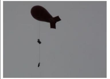
Fig. 10-5 A picture of the tethered balloon. Attached to the string are cloud droplet sampler, condensation nuclei counter, aerosol counter, and radiosonde.
