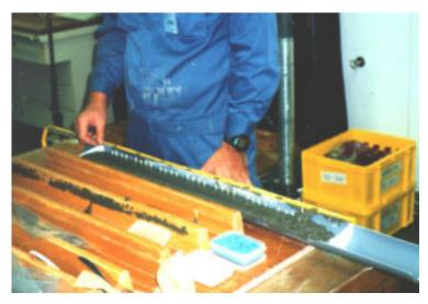
Figure 5. Measurement and insertion of plastic pins in the sediment at 2 cm intervals to mark depth.
