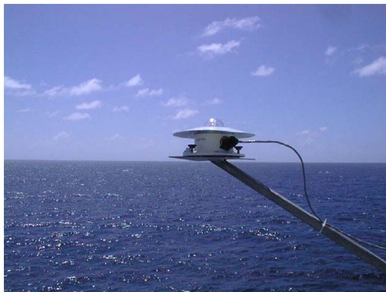
Figure 9. Solar radiation sensor
