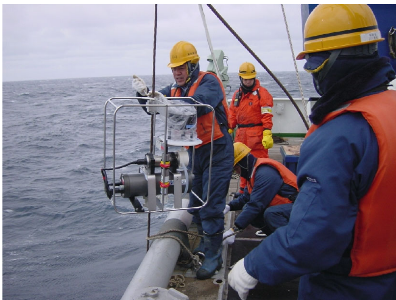
Photo 3.4-1 Deployment of LVP
