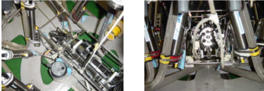
PLATE 2.2.1: PHOTOS OF MOORED CTDs ATTACHED TO THE CTD/RMS FRAME.
