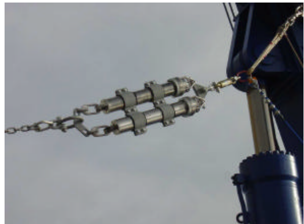
PLATE 2.1.1: PHOTOS OF A MOORED CTD AND ACOUSTIC RELEASERS.
