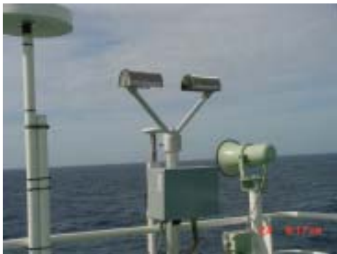
Fig. 7.9-1 Look of the Parsivel M300 sensor installed over the anti-rolling system on the navigation deck.
