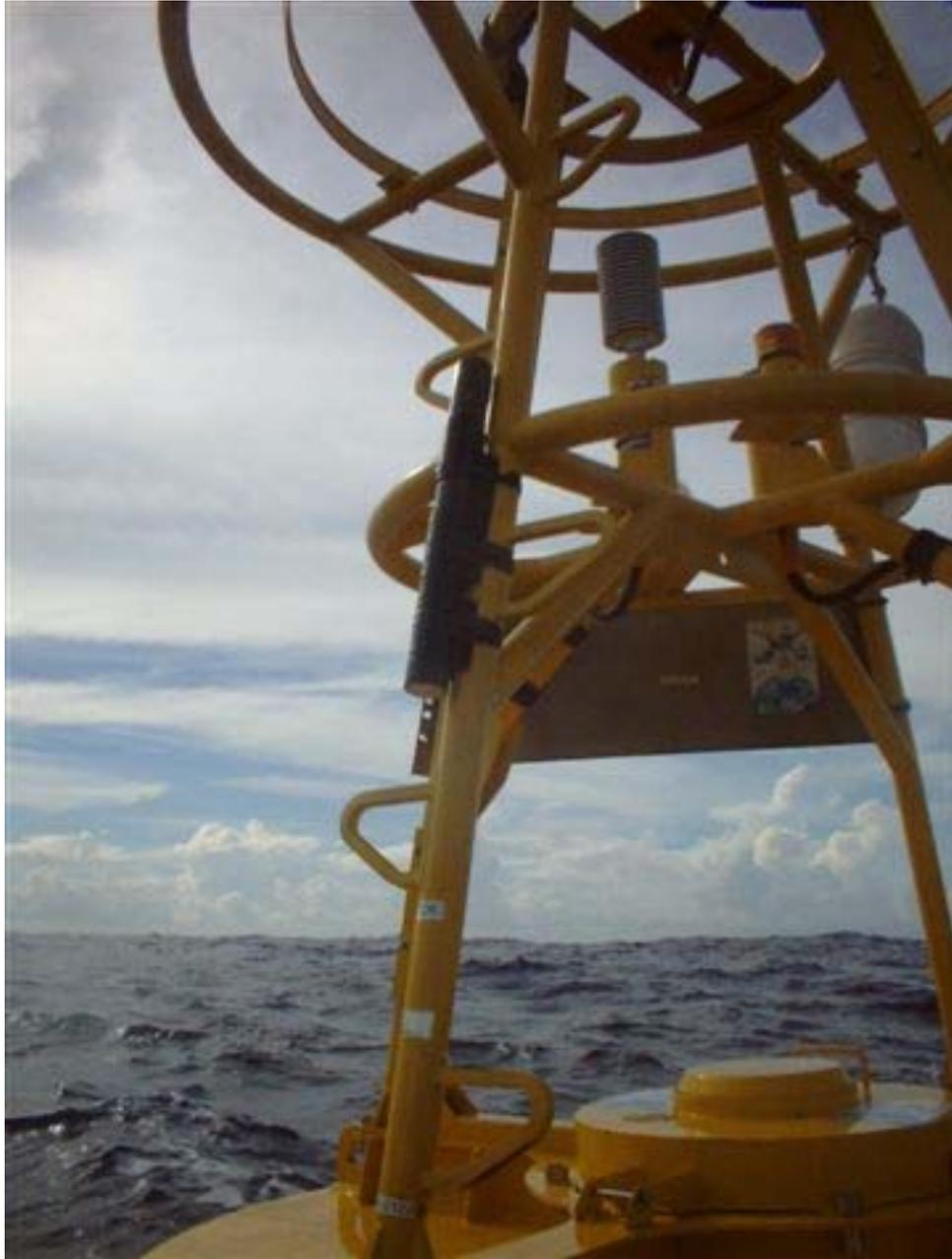
fig.1 Attached ARGOS transmitter
