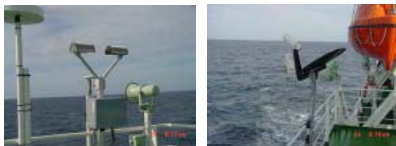
Fig. 7.5.3-1 Look of the Parsivel M300 (left panel) and MRR-2 (right panel) sensors installed on the vessel.
