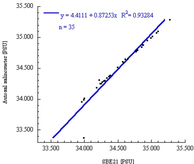
Fig.6-4-1. Comparison between the salinity values measured by SBE21of the Sea Surface Monitoring System and Autosal salinometer for 35 samples.
