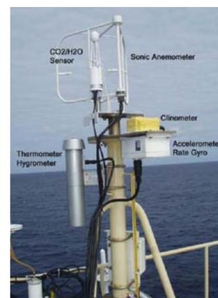
Fig. 7.8-1 Turbulent flux measurement system on the top deck of foremast.
