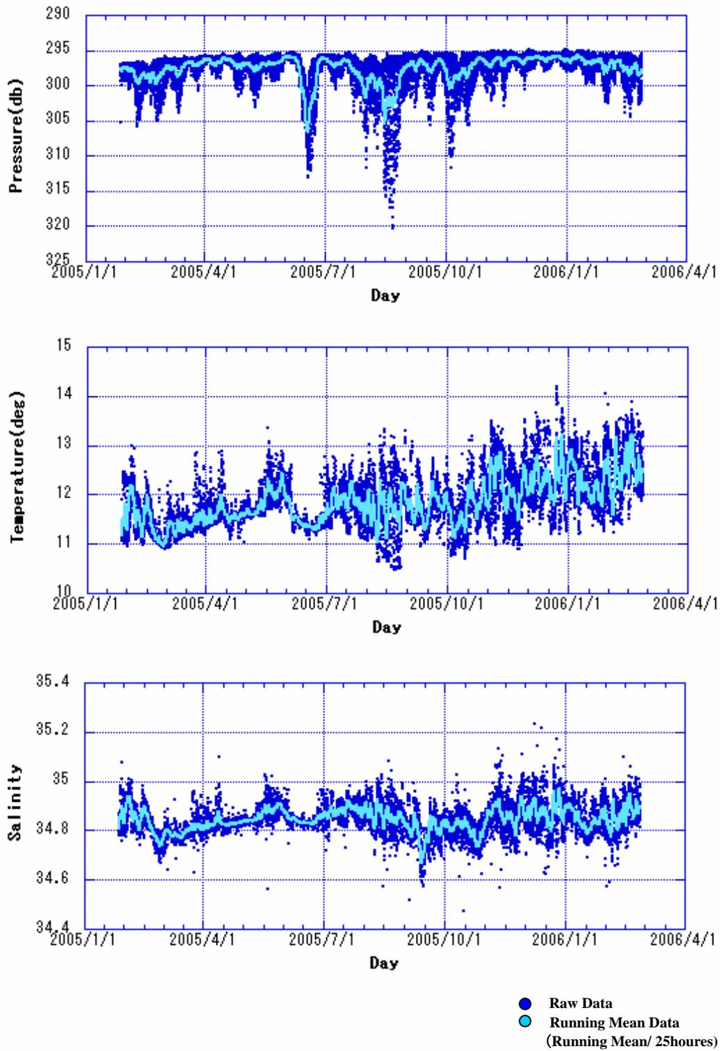
Fig.7-2-3 Time Series of pressure, temperature, salinity of obtained with CTD of EQ-147E mooring (2005/1/27-2006/2/28)
