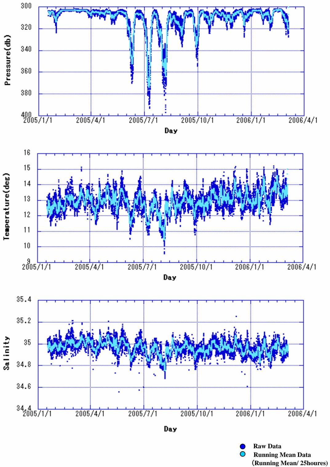
Fig.7-2-5 Time Series of pressure, temperature, salinity of obtained with CTD of 2.5S-142E mooring (2005/1/18-2006/3/7)
