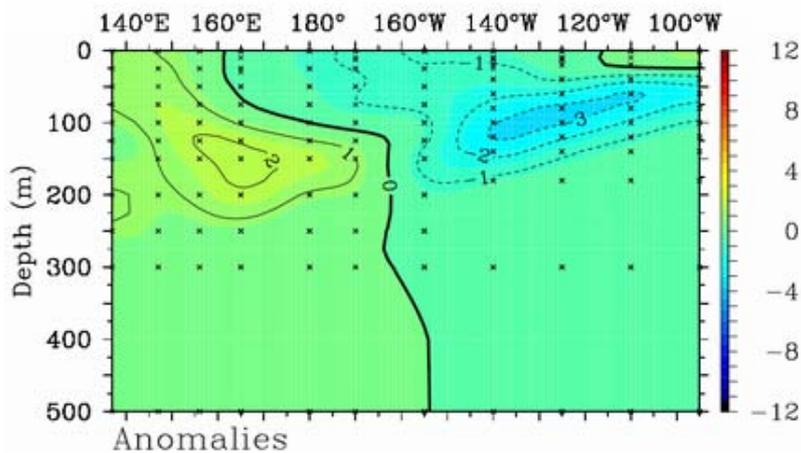
Figure 2-3. Vertical section of temperature anomaly along the equator on February 2006 obtained from TAO/TRITON array.
