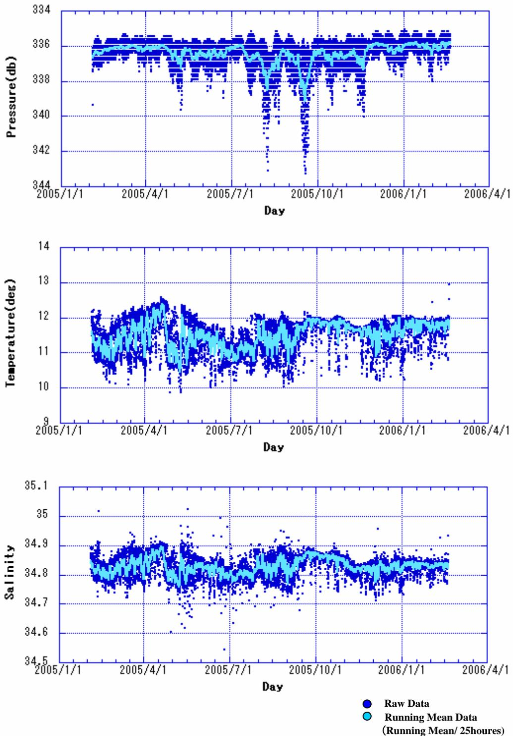
Fig.7-2-2 Time Series of pressure, temperature, salinity of obtained with CTD of EQ-156E mooring (2005/2/4-2006/2/20)
