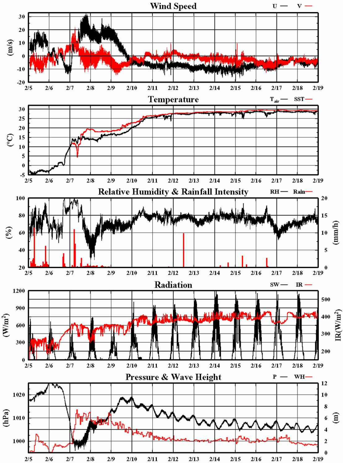
Fig.6.1-1 Time series of surface meteorological parameters during the MR06-01 cruise
