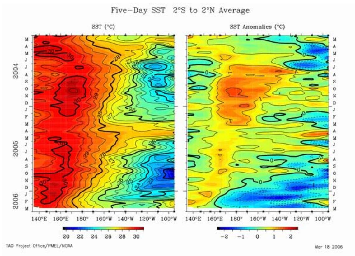
Figure 2-1. Time-longitude plot of sea surface temperature and its anomaly at the equator obtained from TAO/TRITON buoy array from March 2004 to March 2006. (<http://www.pmel.noaa.gov/tao/jsdisplay/>)
