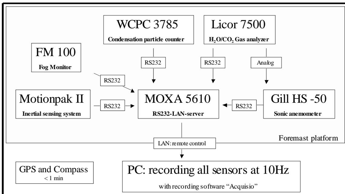
**Figure 6.2.7.2. Technical layout of the EC-System**
