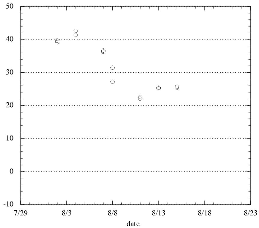
Fig.6.4.2.12 Difference in value between dissolved oxygen sensor and bottle data (Leg.1).
