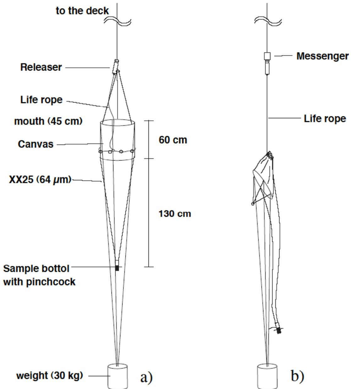
Figure 6.6.1.1 Schematic illustration of the closing net. a) Before closing; b) After closing
