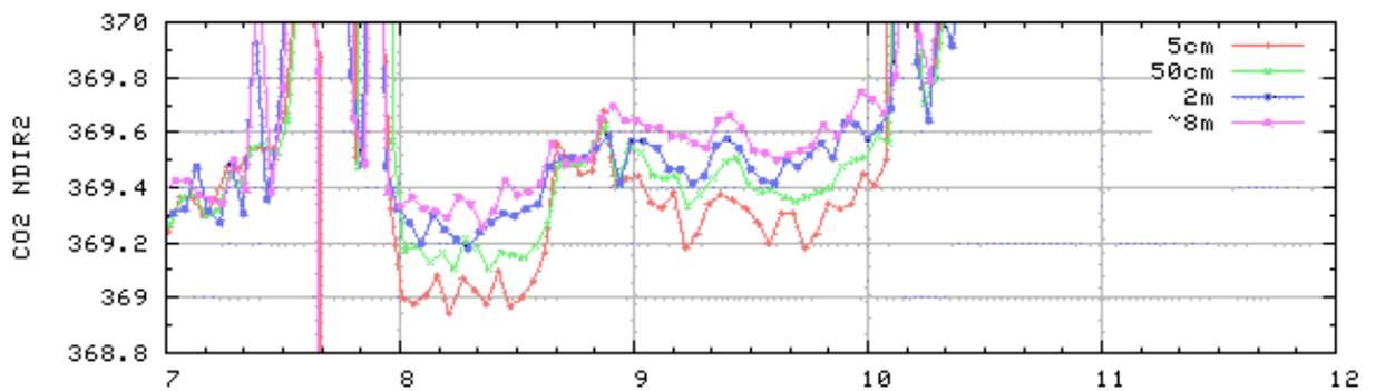
Figure 6.2.9.3 Time variations of CO<sub>2</sub> concentration for 4 levels (5, 50, 200 and 710 cm) at St.13 from 800 till 1000 on Sep. 1<sup>st</sup> 2006.
