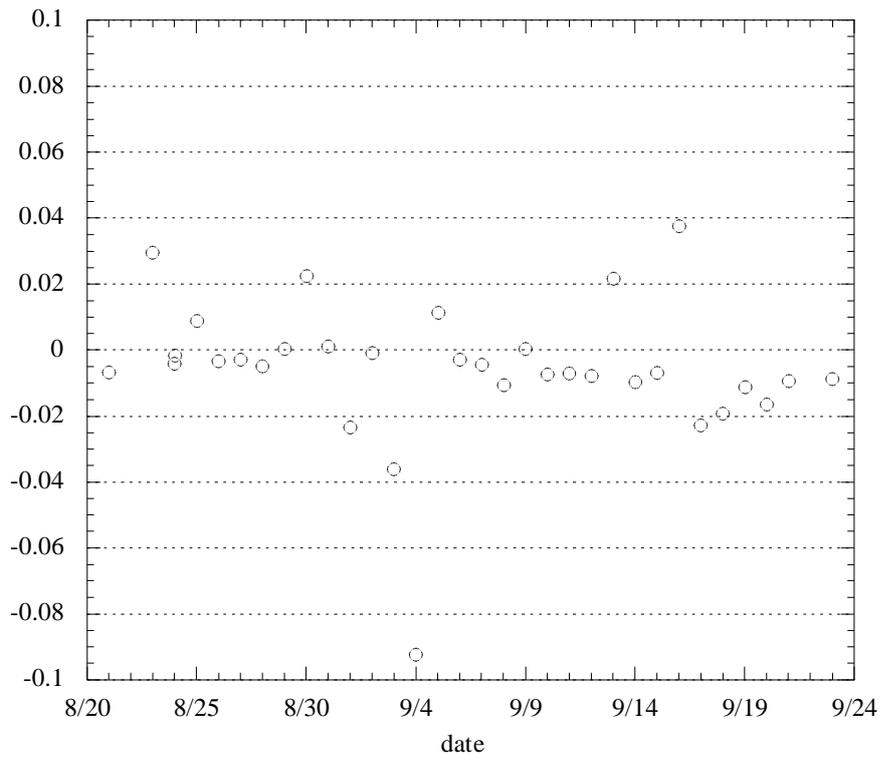
Fig.6.4.2.14 Difference in value between salinity sensor and bottle data (Leg.2).
