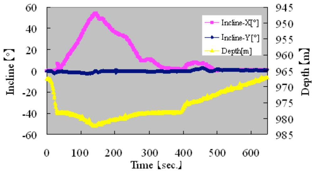
Figure 6.8.2.2 The performance when the core barrel of piston corer was bended (Core Name: PC-01-B).
