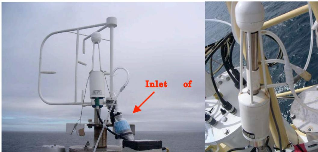
Figure 6.2.5.1 The installation of the turbulence measurement sensors and inlet of sample gas (left panel), and a sealed-up LI7500 (right panel).
