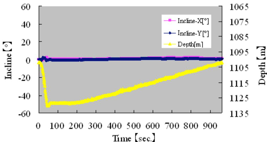
Figure 6.8.2.1 The performance when piston corer plumbed down and core barrel penetrated into sea floor (Core Name: PC-06-R).
