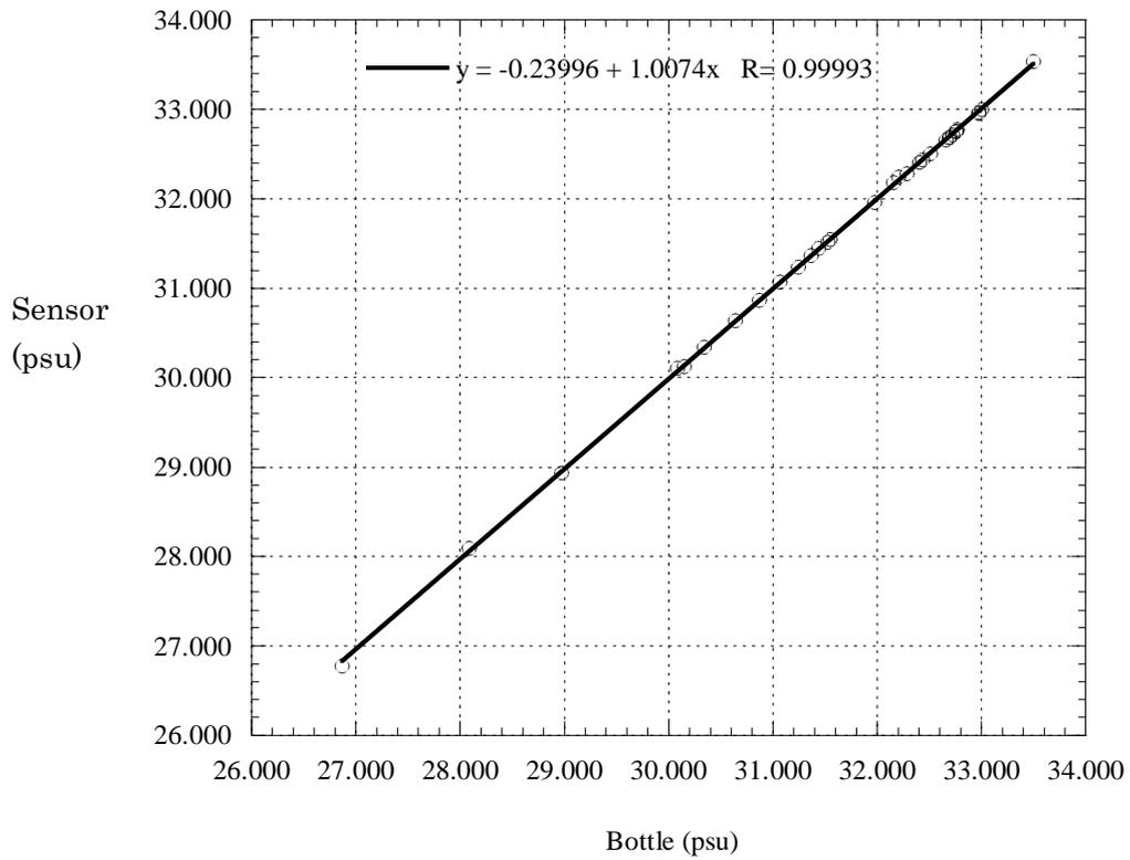
Fig.6.4.2.13 Comparison between salinity sensor and bottle data (Leg.2)
