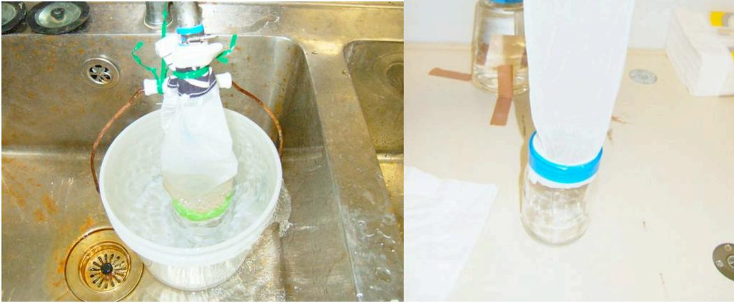
Figure 6.6.2.1 Surface water filtration (left) and the filtration apparatus (right)
