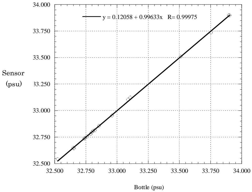
Fig.6.4.2.9 Comparison between salinity sensor and bottle data (Leg.1)
