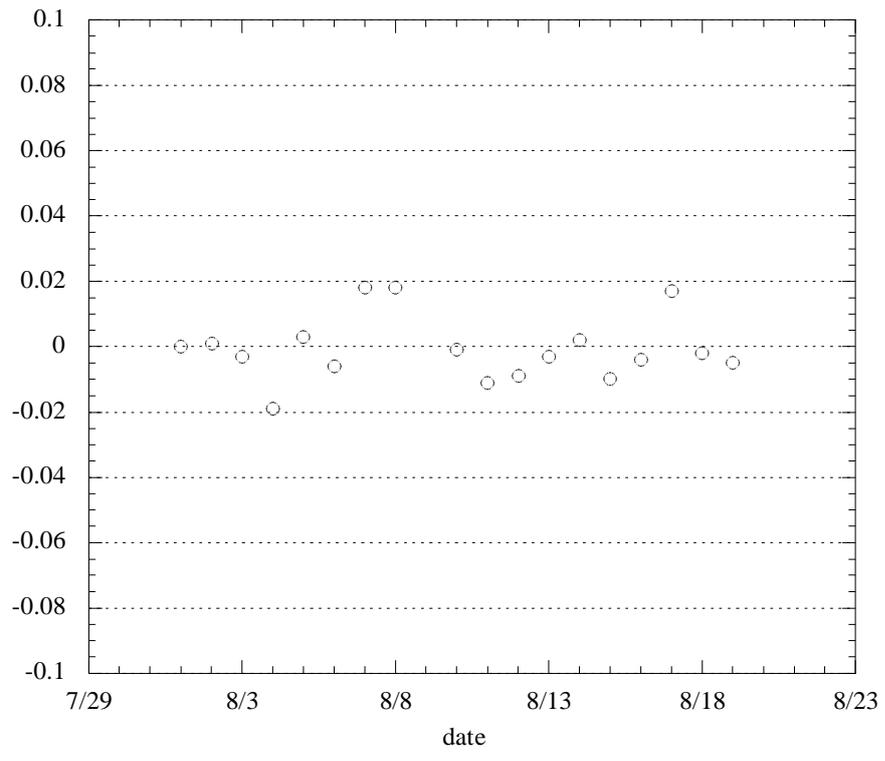
Fig.6.4.2.10 Difference in value between salinity sensor and bottle data (Leg.1).
