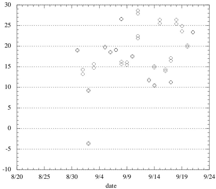
Fig.6.4.2.16 Difference in value between dissolved oxygen sensor and bottle data (Leg.2).
