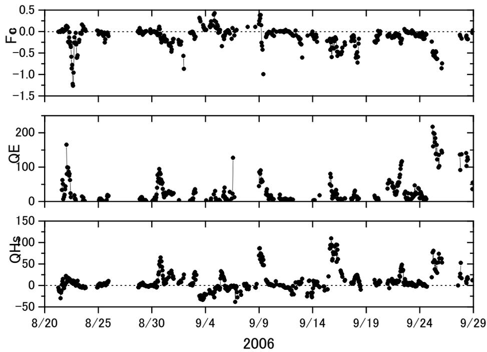
Figure 6.2.5.2 Preliminary results of eddy fluxes of sensible heat (QHs), latent heat(QE) and CO<sub>2</sub>(Fco) calculated with eddy-covariance method. The sensible heat flux and the latent heat flux were given in W m<sup>-2</sup> and CO<sub>2</sub> flux is given in mgCO<sub>2</sub> m<sup>-2</sup> s<sup>-1</sup>. Corrections were not applied to the sensible heat flux (QHs) for water vapor contribution, and to the CO<sub>2</sub> flux (Fco) for the Webb correction.
