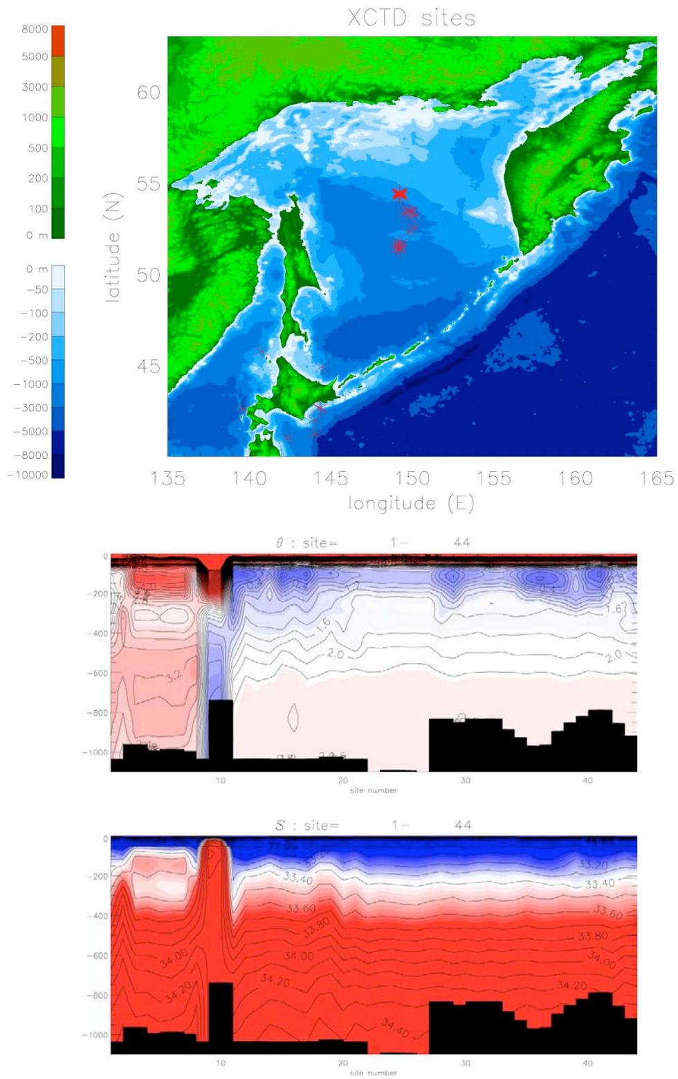
Figure 6.3.1.1: (Upper) The locations of XCTD stations and (lower) the vertical sections of potential temperature and salinity along the ship track.
