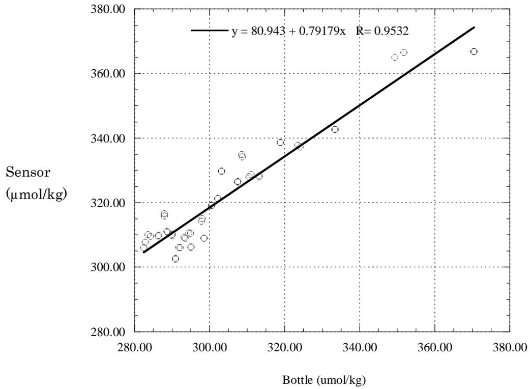
Fig.6.4.2.15 Comparison between dissolved oxygen sensor and bottle data (Leg.2).
