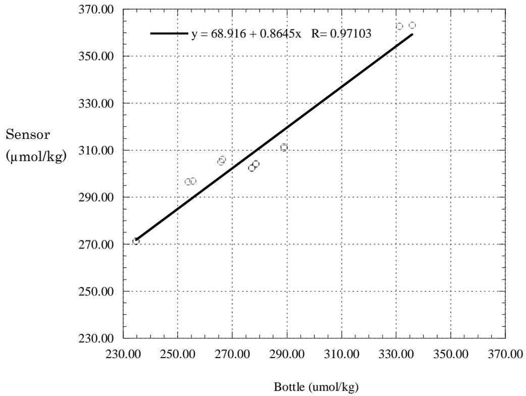
Fig.6.4.2.11 Comparison between dissolved oxygen sensor and bottle data (Leg.1).
