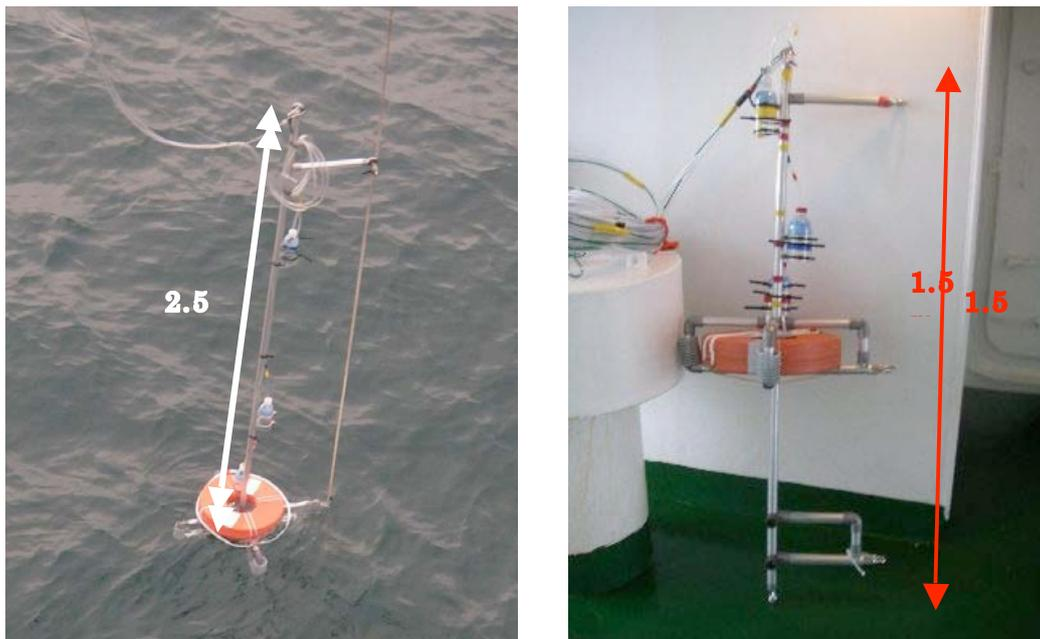
Figure 6.2.9.2 Buoys for gas sampling for fine condition (a) and for rough condition (b).
