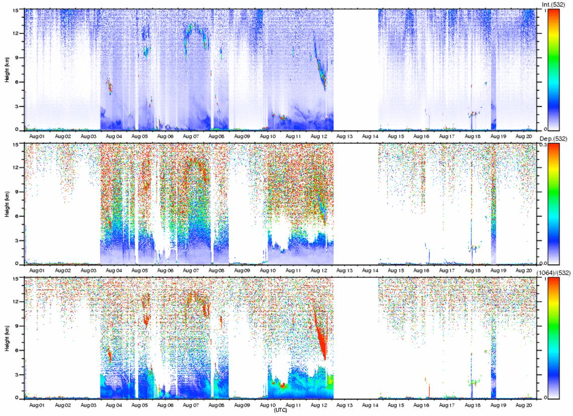
Figure 6.2.4.1 Time-height indications of backscattering intensity at 532 nm (top), depolarization ratio at 532 nm (middle), and ratio of backscattering intensities between 1064 nm and 532 nm (bottom), during MR06-04 leg 1. Depolarization ratio is a measure of non-sphericity of particles, and ratio of two wavelengths is a measure of particle size.
