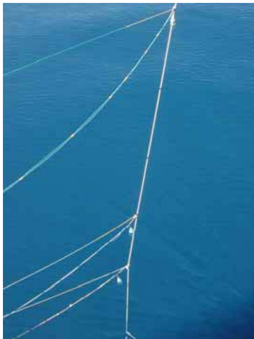
Fig. 5.17-2. Lower three inlets of sample gas at the head of the ship.
