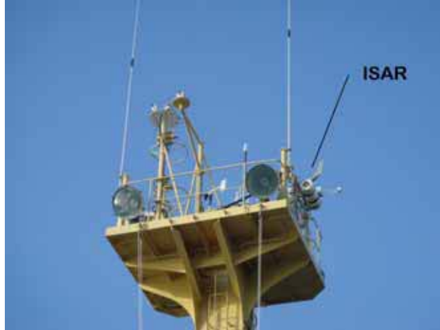
Fig. 5.14.1-1. The ISAR (Infrared Sea Surface Temperature Autonomous Radiometer) was mounted on the foremast, starboard side with a 45° view to the ocean.
