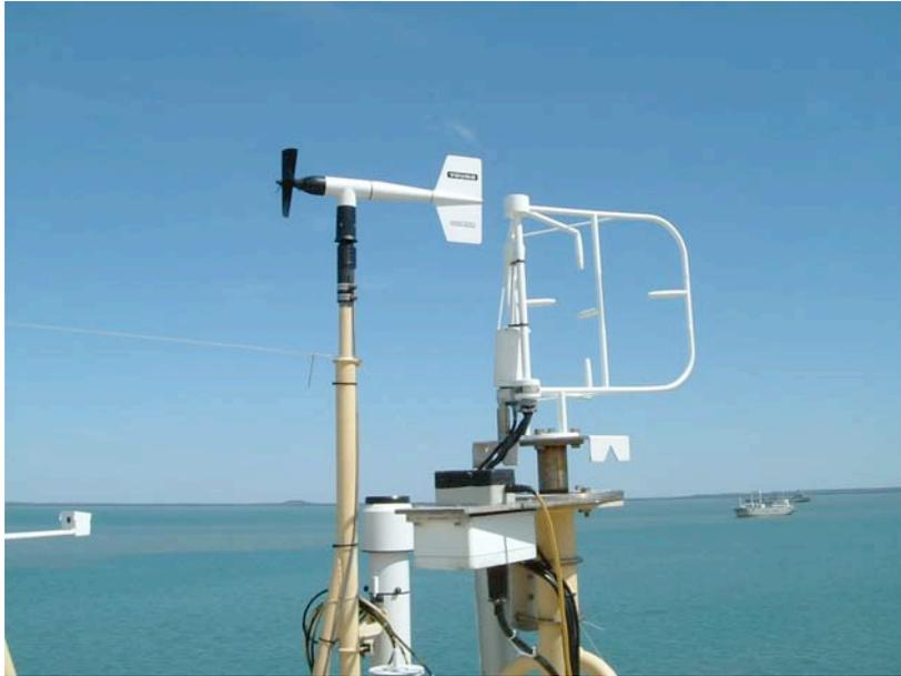
Fig.1. Installation of the turbulent flux and ship motion correction systems on the top of the foremast.
