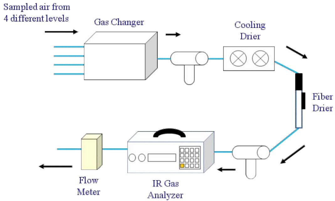
Fig.1 CO<sub>2</sub> profile measurement system
