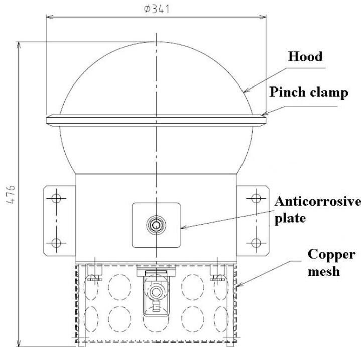
Fig. 1. Side view of pCO<sub>2</sub> sensor.
