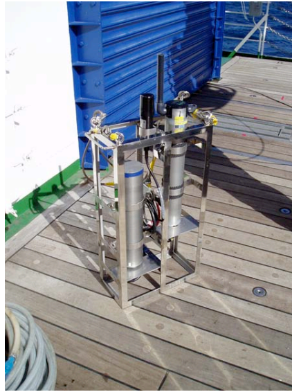
Fig. 1. FRR fluorometer (Diving Flash, Kimoto Electric Co., Ltd., Japan).
