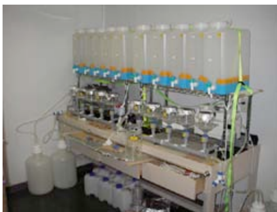
Figure 1. Photograph of large volume filtration system.
