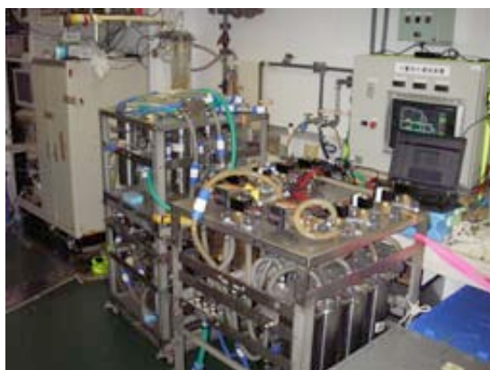
Figure 2. Mega volume filtration system setting up in the surface sea-water analysis room in “MIRAI”. The equipment is consist of a) steel-wool parts, b) 10 \mu\text{m} size filter parts, c) 1.0 \mu\text{m} size filter parts, d) 0.5 \mu\text{m} size filter parts, e) 0.2 \mu\text{m} size filter parts, and f) control units (control panel and data logger PC). The maximum filtration velocity is about 10 L/min.
