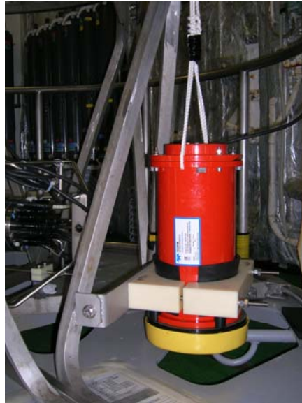
Fig 7.4-1 Mounting of LADCP on CTD System
