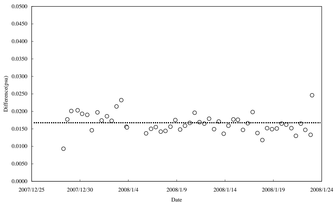
Fig.6.4-2 Variability of difference between sensor data and bottle data in salinity. The mean of the difference was 0.0165psu.
