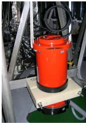
Figure 7-3-1. Mounting of LADCP on the CTD System
