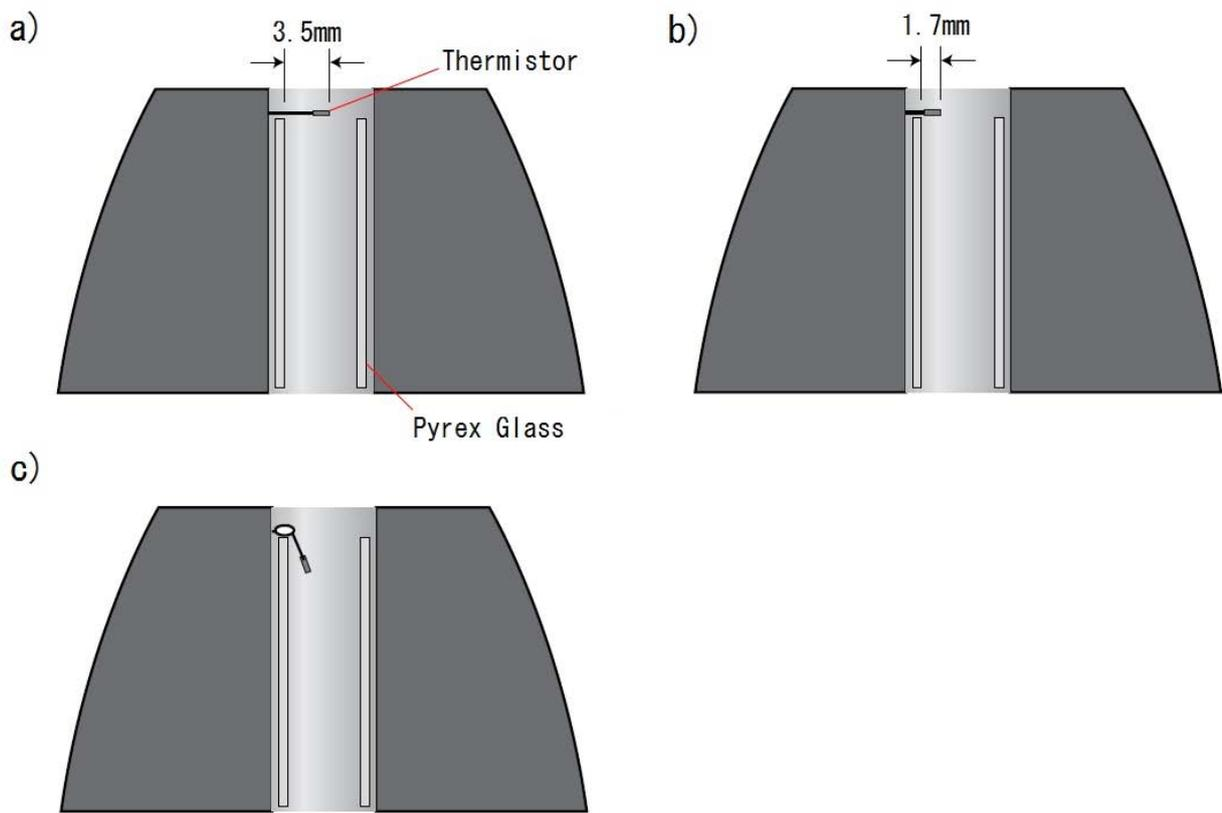
Figure 7-14-2. Structure of head of XCTD probes. a) Long, b) Short, and c) Bended-type, respectively.
