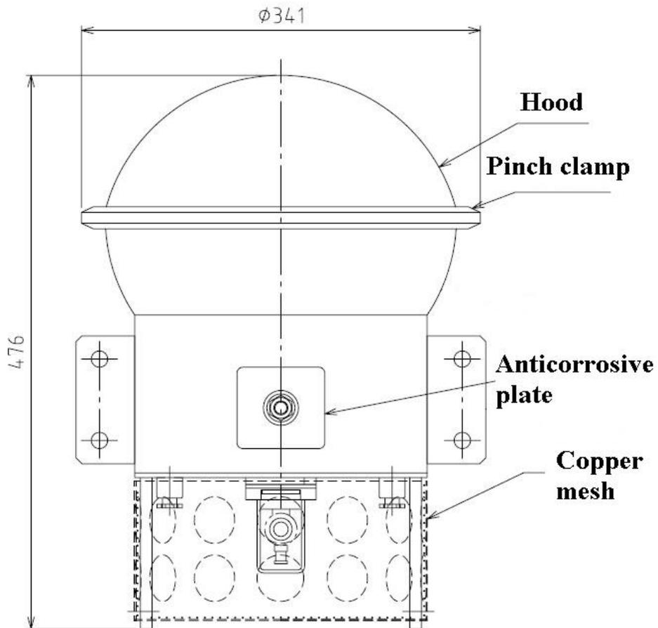
Fig. 7.5-1 Side view of pCO<sub>2</sub> sensor.
