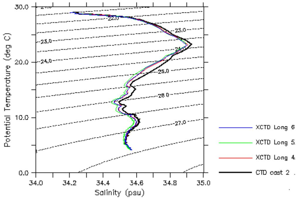
XCTD test (CTD-2 vs XCTD-L)
