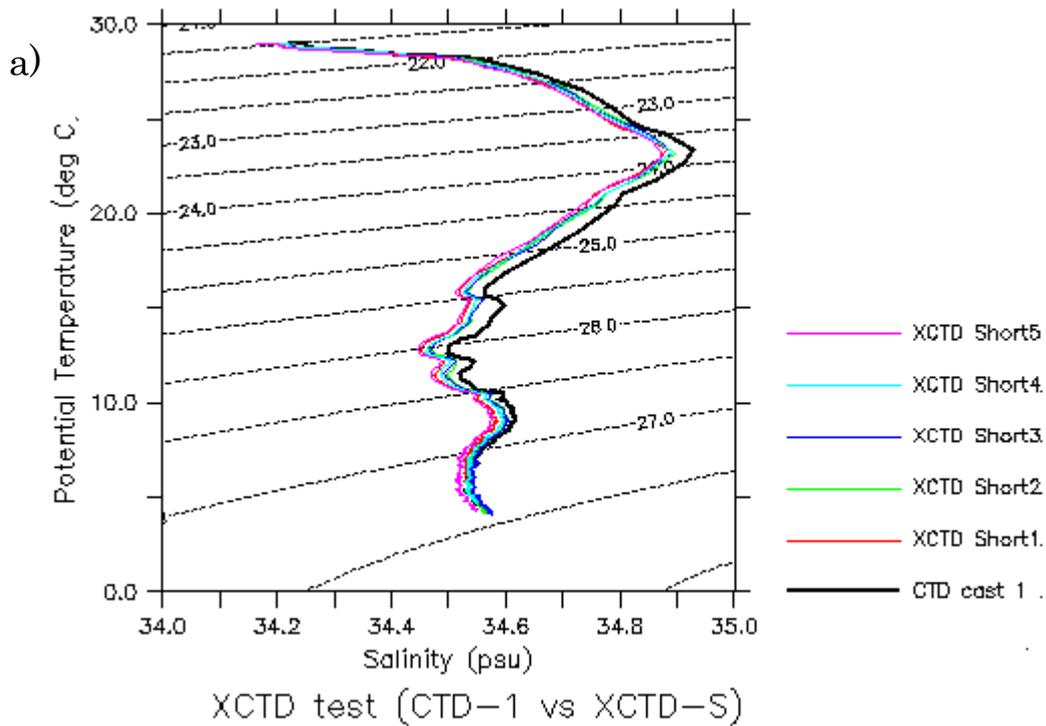
Figure 7-14-3. Potential temperature - salinity relations in the XCTD performance test. Results from a) CTD cast 1 versus Short-type XCTD probes, b) CTD cast 1 versus Long-type probes 1-3, c) CTD cast 2 versus Bended-type probes, d) CTD cast 2 versus Long-type probes 4-6, and e) average of two CTD cast versus averages of Short, Bended, and Long type probes, respectively.
