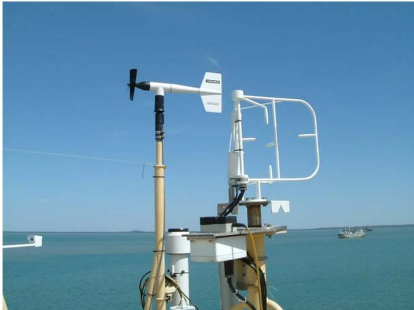
Fig.7.7-1. Installation of the turbulent flux and ship motion correction systems on the top of the foremast.
