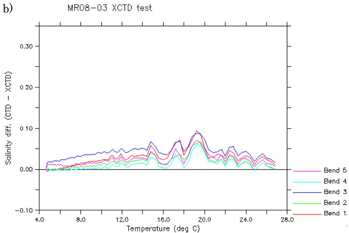
Figure 7-14-4. Graphs of CTD salinity minus XCTD salinity for temperature in this test. Results from a) Short-type XCTD probes, b) Bended-type probes, c) Long-type probes, and d) averages of these three type probes, respectively.
