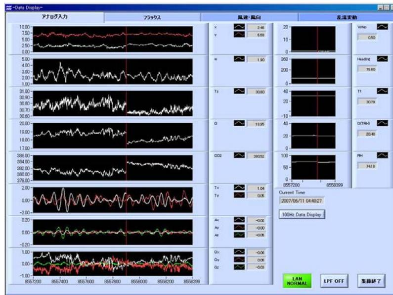
Fig.7.7-2. PC-based real time logging and monitoring system using LabVIEW8 software.
