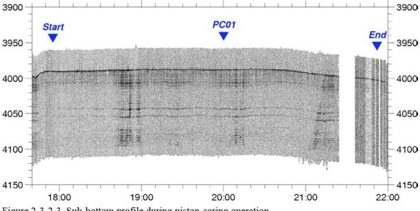
Figure 2-3-2-3. Sub-bottom profile during piston-coring operation.
