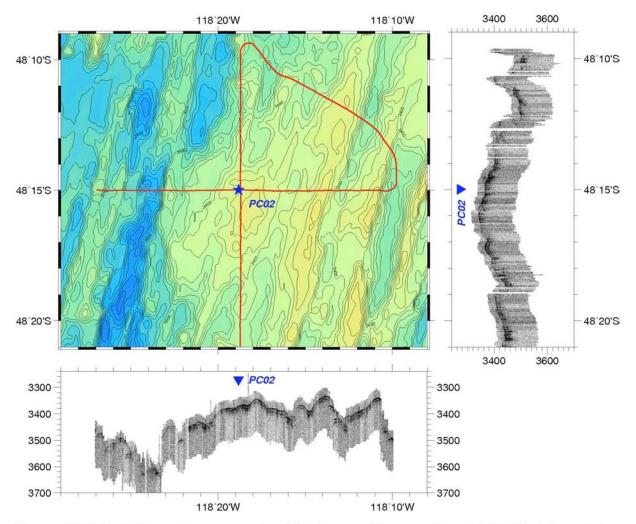
Figure 2-3-2-5. Bathymetric map and sub-bottom profiles crossing site PC02 taken during single-channel seismic reflection survey.
