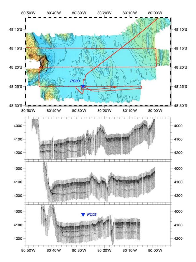
Figure 2-3-2-7. Bathymetric map with survey lines, and sub-bottom profiles around the site PC03.
