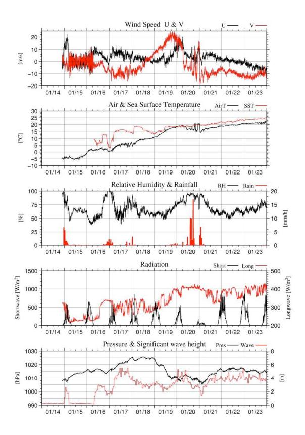
2-7-1-Fig1 Time series of surface meteorological parameters during the MR08-06 cruise
