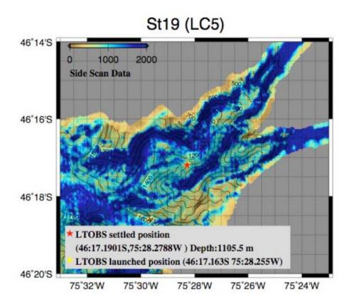
2-4-3-Fig. 4: Locations of the settled LTOBS for St17-21 (LC1-LC5), respectively. Background color shows the intensity of the acoustic reflections from the seafloor by the Side-scan data.
