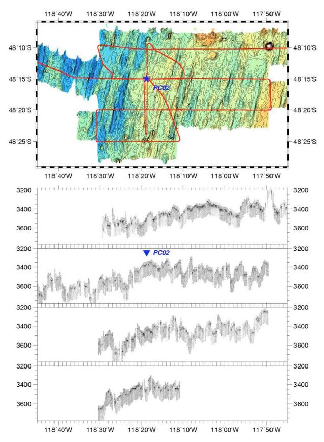
Figure 2-3-2-4. Bathymetric map with survey lines, and sub-bottom profiles around the site PC02.
