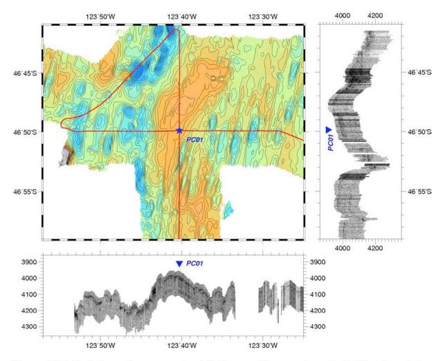
Figure 2-3-2-2. Bathymetric map and sub-bottom profiles crossing site PC01 taken during single-channel seismic reflection survey.
