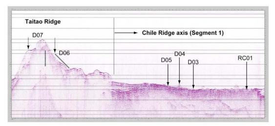
Figure 2-4-5-12: Dredge sites D06 and D07 indicated on the SCS (st27-st30) profile. Position of D06 and D07 is off profile from the NS-trending st27-st30 profile. Latitude of D06 and D07 is indicated by arrow with dashed line. When they are projected to the st27-st30 profile, the position of dredges D06 and D07 correspond to those indicated by oblique and vertical dashed lines, respectively.
