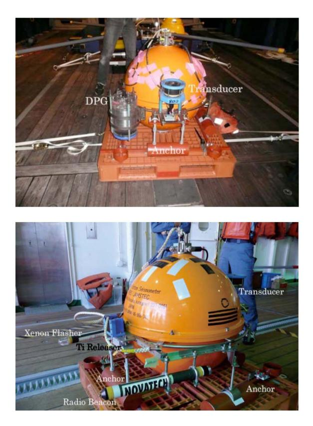
Fig. 1 Appearance of broadband ocean bottom seismometer (BBOBS) deployed at st. 8 (upper) and st. 9 (lower).
