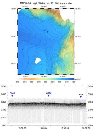
Figure 2-4-6-1: Bathymetric map around site PC04 and sub-bottom profiles during the coring.
