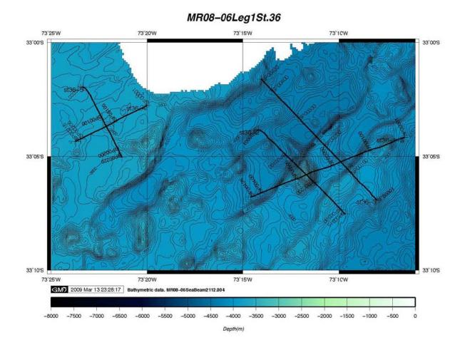
Fig. 2-5-1 Single channel seismic survey lines in the petit-spot VI research area.
