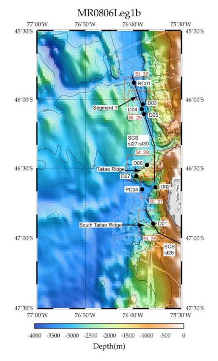
Figure 2-4-5-2: Dredge (D), rock core (RC) and piston core (PC) sites in the Chile Triple Junction area.
