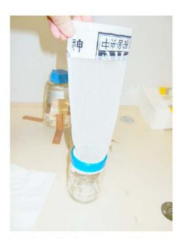
2-6-fig 1 Surface water filtration apparatus consists of 100  $\mu$ m opening mesh and glass bottle.
