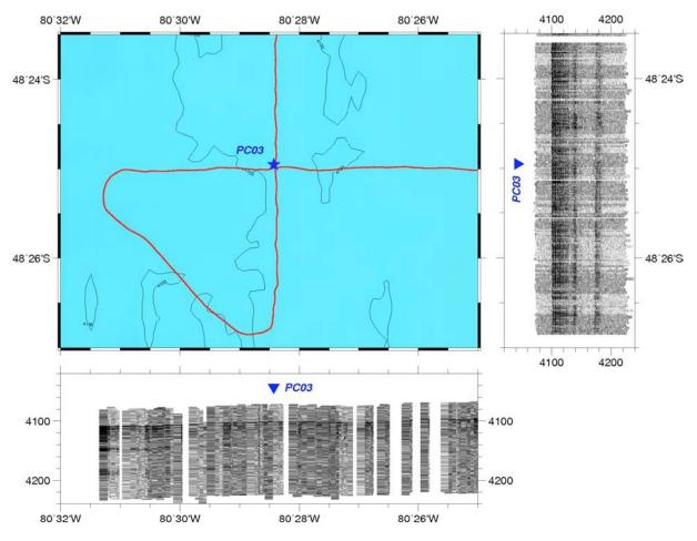
Figure 2-3-2-8. Bathymetric map and sub-bottom profiles crossing site PC03 taken during single-channel seismic reflection survey.
