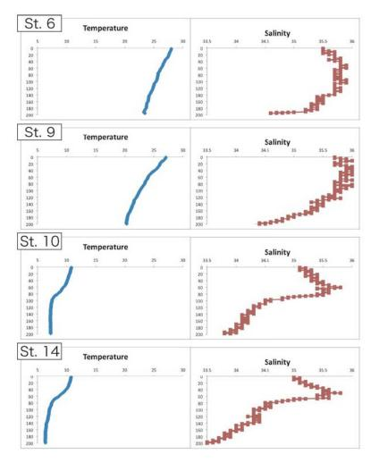
2-6-fig 4 Vertical profiles temperature (left) and salinity (right) at plankton net sampling sites. Data was measured by the CTD logger during plankton net towing.
