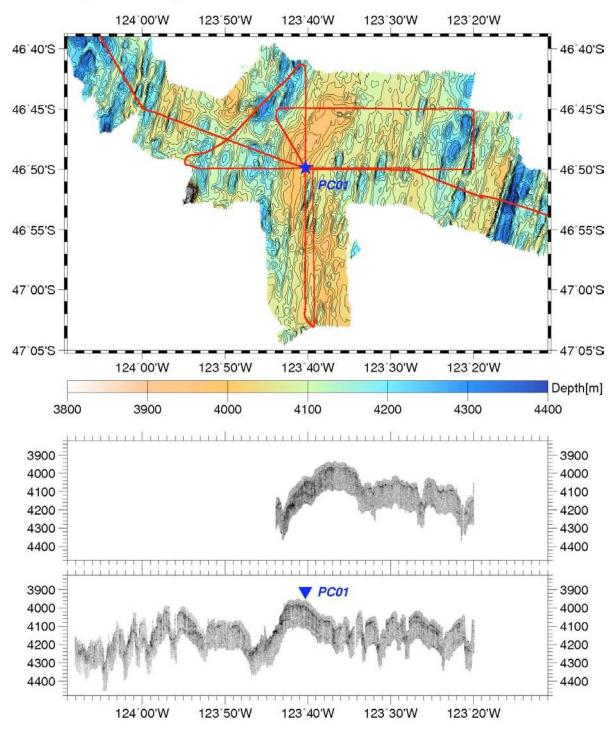
Figure 2-3-2-1. Bathymetric map with survey lines, and sub-bottom profiles around the site PC01.
