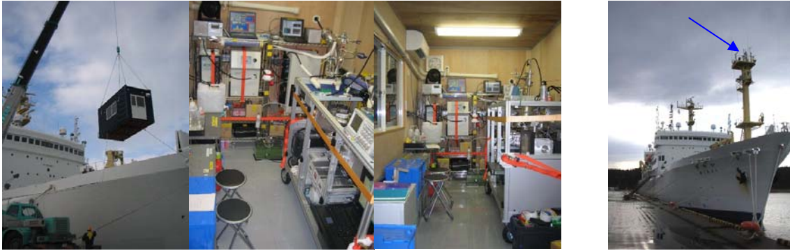
Plate 2.12.1. Installation of a newly constructed container laboratory to #1 storage in R/V Mirai; inside the container laboratory during MR08-06 cruise; air sampling inlet for the instruments in the container laboratory (blue arrow).
