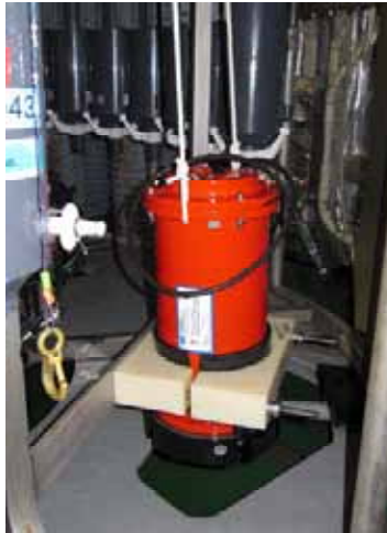
Fig 7-3-1. Mounting of LADCP on the CTD System
