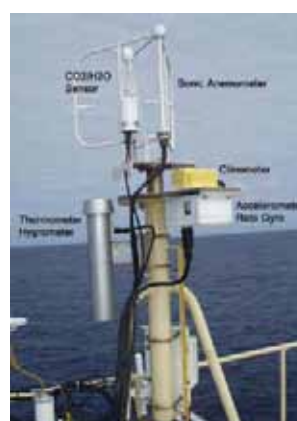
Fig. 7.10-1 Turbulent flux measurement system on the top deck of the foremast.
