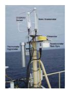
Fig. 2.7-1. Turbulent flux measurement system on the top deck of the foremast.
