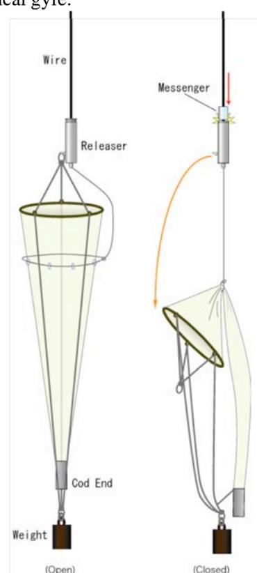
Fig.1 Schematic illustration of closing NORPAC net. Plankton net is open during towing (left), and closed at the top of the sampling depth range by deploying a messenger (right).
