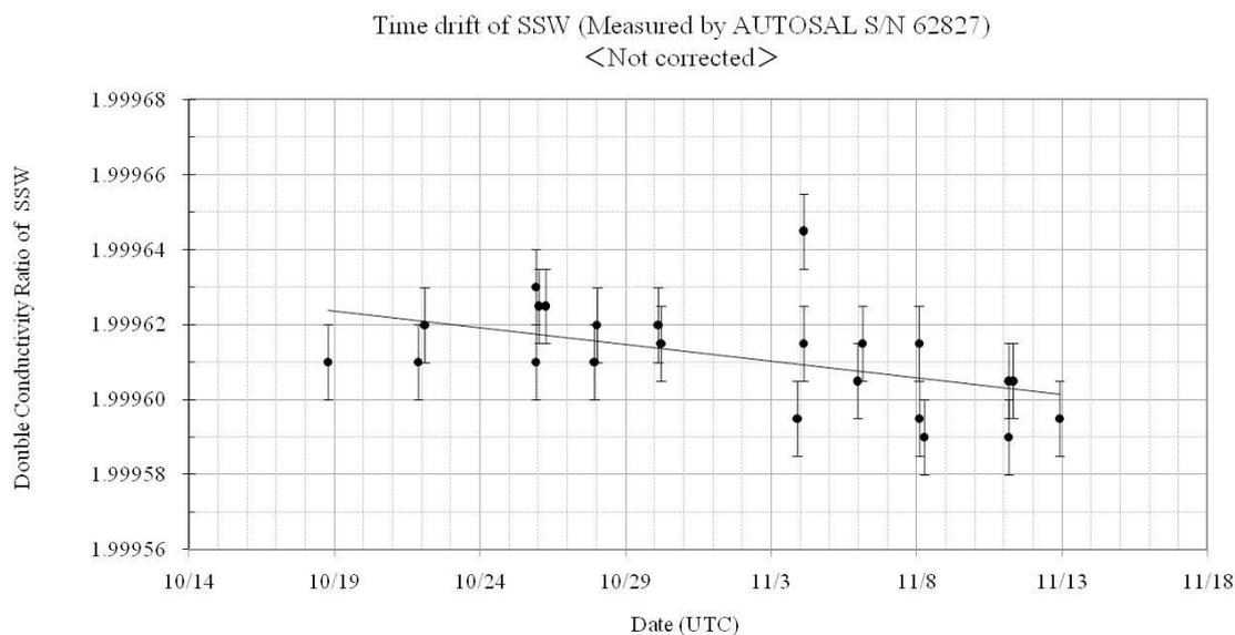
Fig. 2.2.2-1 The history of the double conductivity ratio for the Standard Seawater batch P152(Before correction)
