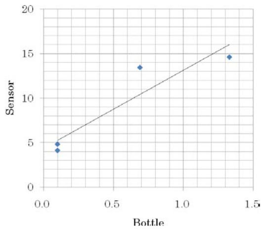
Fig. 2.3-4. Correlation of fluorescence between sensor data and bottle data.
