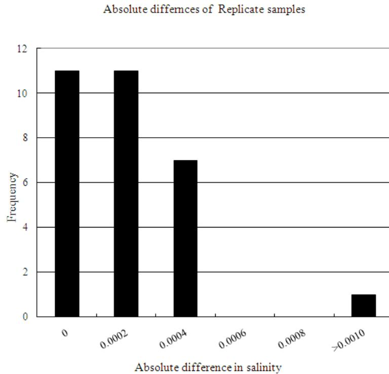
Fig. 2.2.2-3 The histogram of the double conductivity ratio for the absolute difference of replicate samples
