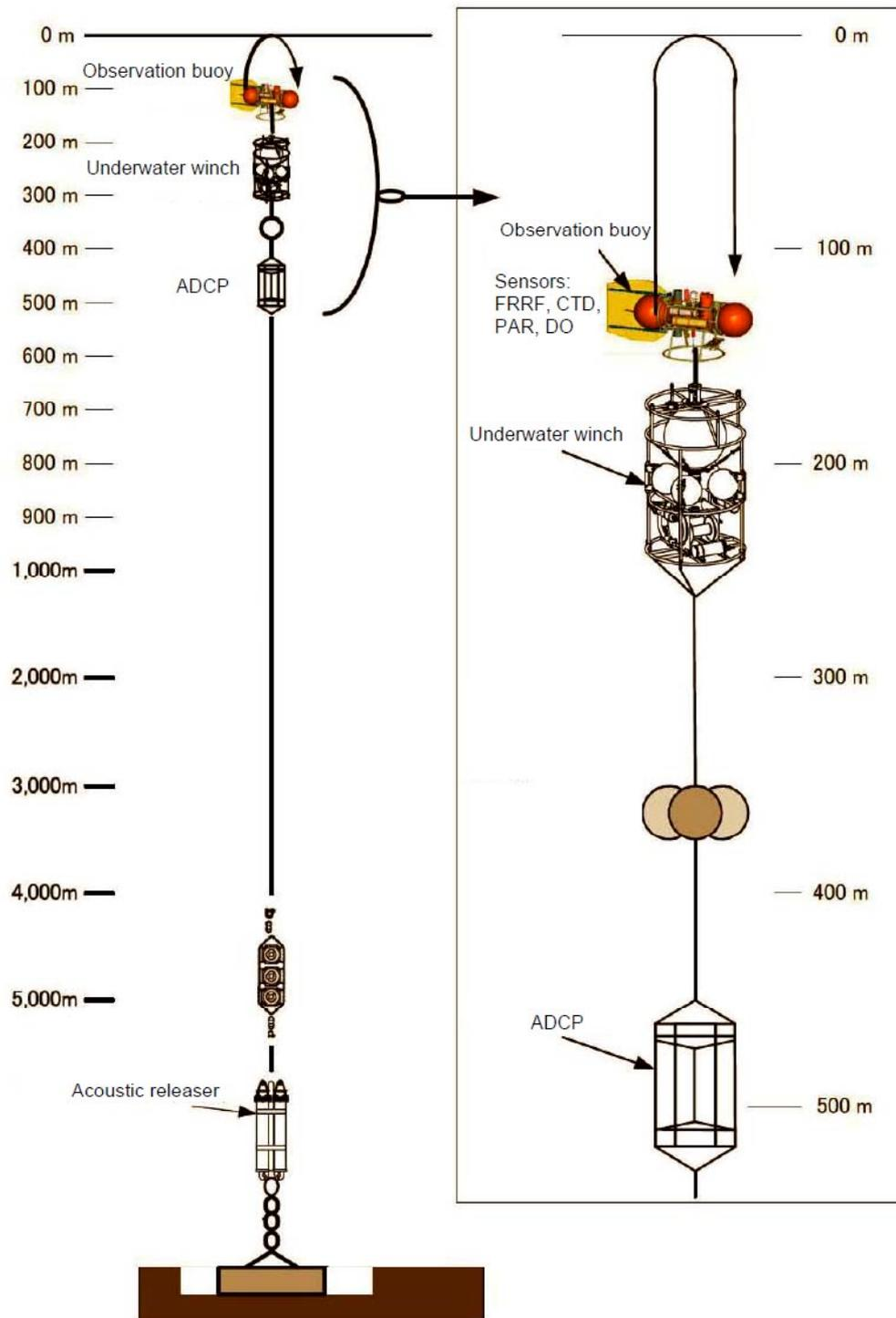
Figure 1a. Schematic diagram of the primary productivity profiler.
