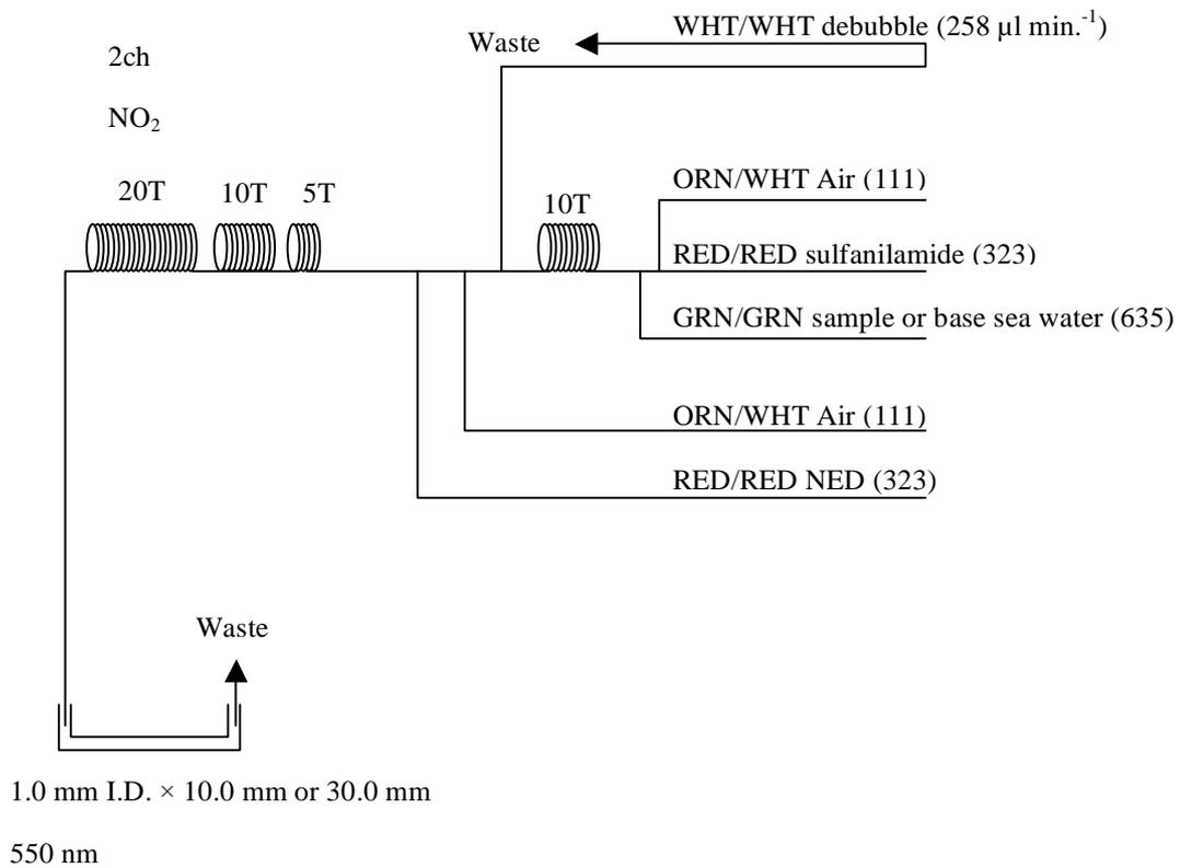
Figure 2.5.3 NO<sub>2</sub> (2ch.) Flow diagram.
