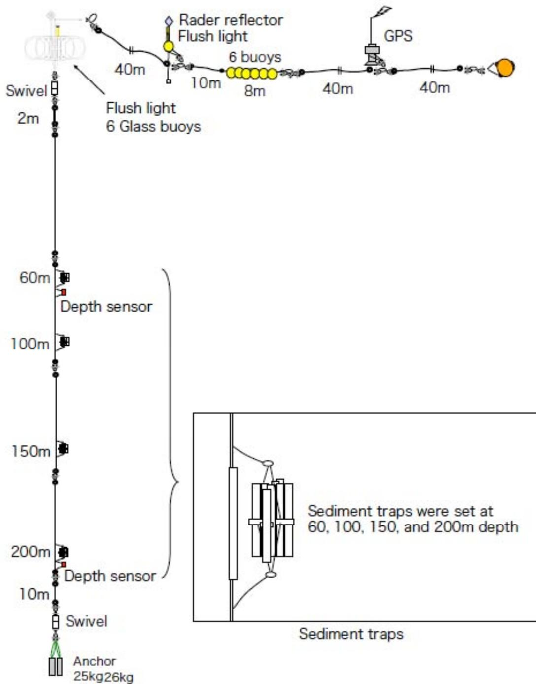
Fig. 3.5.1-1 Drifting mooring system at stations K2 and S1.
