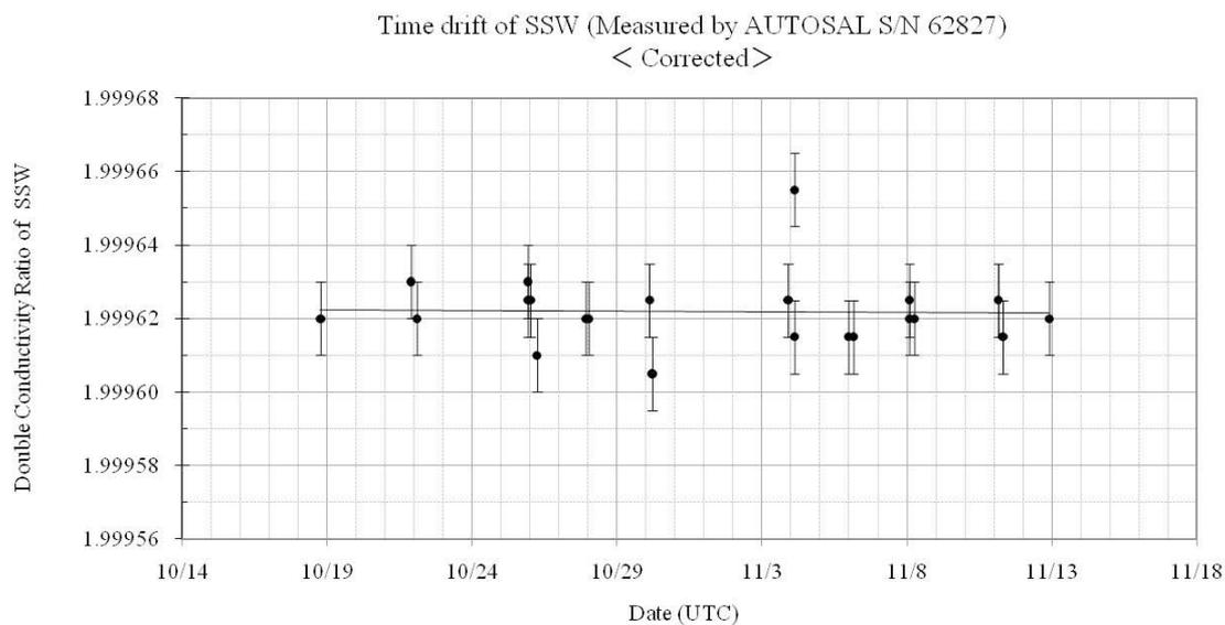
Fig. 2.2.2-2 The history of the double conductivity ratio for the Standard Seawater batch P152(after correction)
