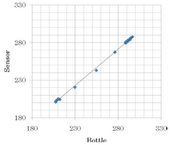
Fig. 2.3-3. Correlation of dissolved oxygen between sensor data and bottle data.
