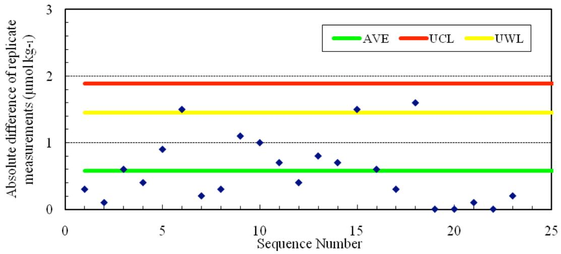
Figure 2.8-1 Range control chart of the absolute differences of replicate measurements carried out in the analysis of TA during the MR10-06 cruise. UCL and UWL represents the upper control limit ( $UCL=AVE*3.267$ ) and upper warning limit ( $UWL=AVE*2.512$ ), respectively.
