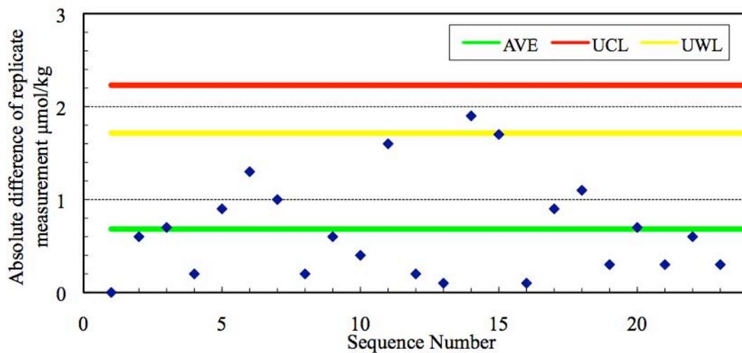
Figure 2.7-1 Range control chart of the absolute differences of replicate measurements of DIC carried out during this cruise. UCL and UWL represents the upper control limit ( $UCL = AVE * 3.267$ ) and upper warning limit ( $UWL = AVE * 2.512$ ), respectively.
