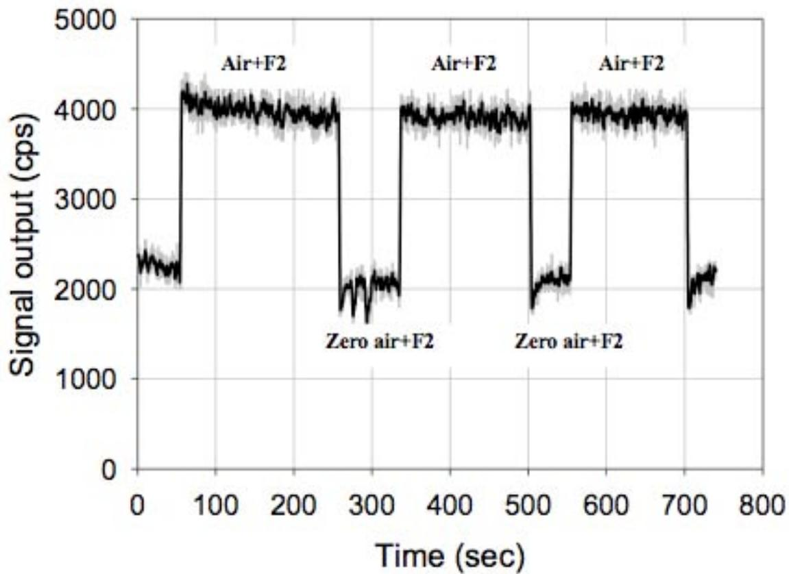
Figure 3. Photon signals emitted from chemiluminescence of sample air and zero gas with  $F_2$ . Gray line is the raw data obtained at every 0.1 sec, and thick black line is the data obtained by 1 sec -running mean. The difference the signals between those from reaction of air with  $F_2$  and those from reaction of zero air is probably attributed to the reaction of DMS with  $F_2$ .
