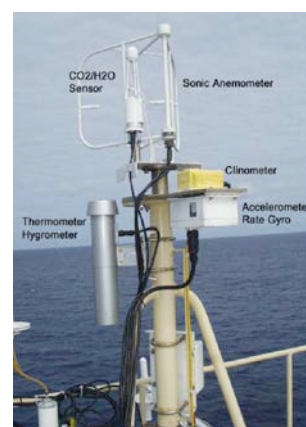
Fig. 1 Turbulent flux measurement system on the top deck of the foremast.
