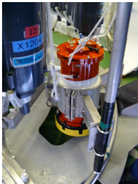
Fig 7.4-1 Mounting of LADCP on CTD System (photo: S. Soares)
