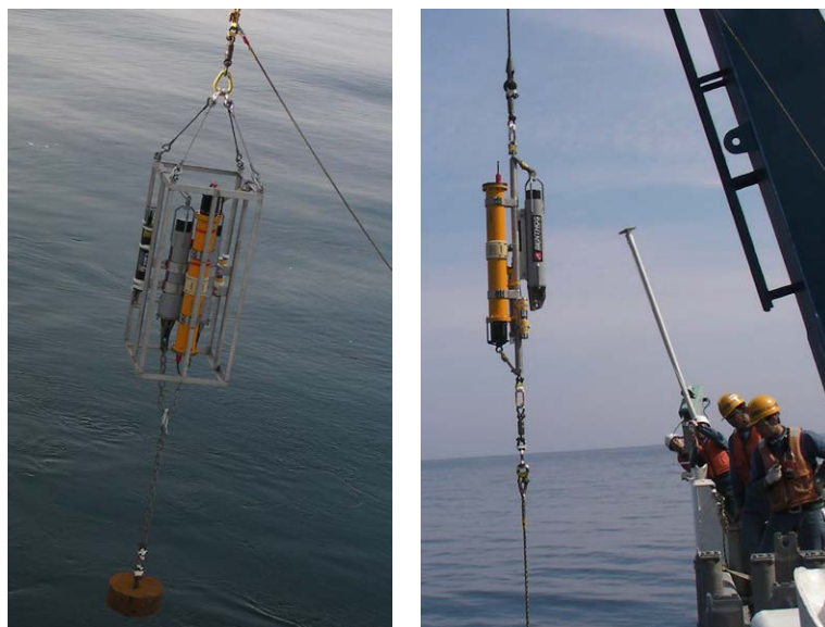
Fig.3 Photos of a bottom station (left) and a buoy station (right).
