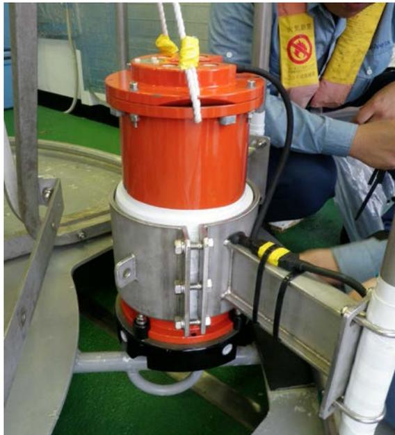
Fig 7.4-1 Mounting of LADCP on CTD System (photo: Y. Kashino)
