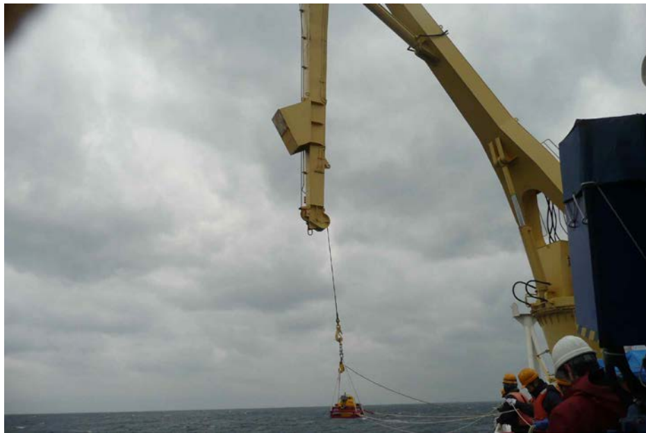
Fig. 5.3.1 Installation operation by multi-joint crane on R/V Mirai
