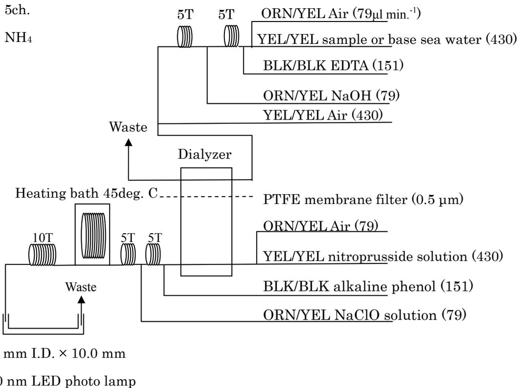
Figure 4.2.6 NH<sub>4</sub> (5ch.) Flow diagram.
