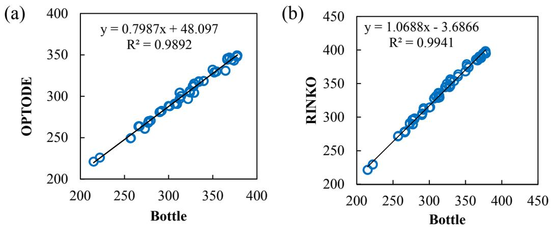
Fig 4.3-3 Correlation of dissolved oxygen between sensor data and bottle data.
