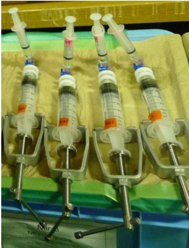
Fig. 4.14.2-1. System of squeezing pore water from sediment samples
