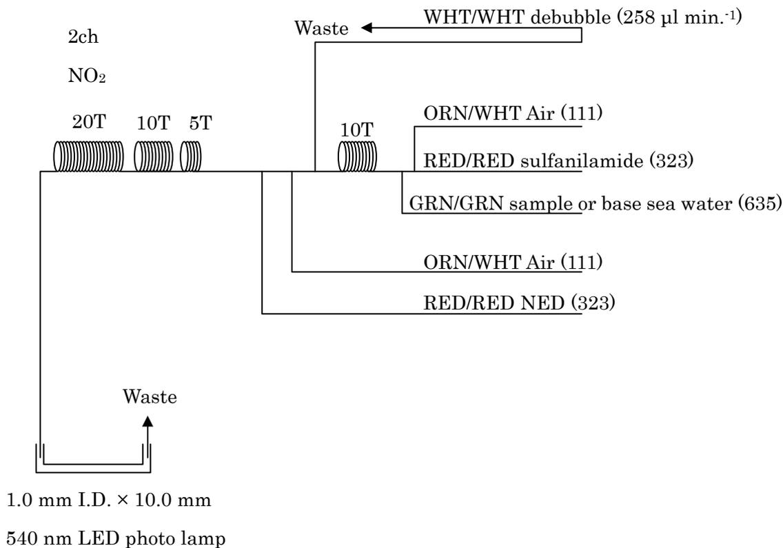
Figure 4.2.3 NO<sub>2</sub> (2ch.) Flow diagram.
