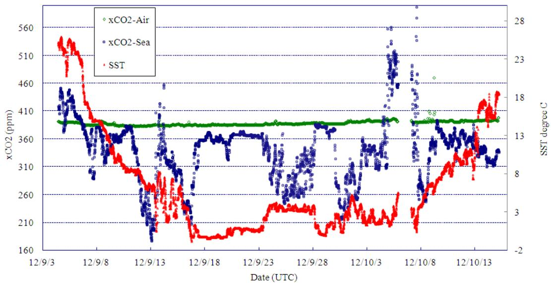
Figure 4.4-2 Time series of atmospheric and oceanic CO<sub>2</sub> concentration (xCO<sub>2</sub>). Green dots represent atmosphere xCO<sub>2</sub> variation and blue oceanic xCO<sub>2</sub>. SST variation (red) is also shown.
