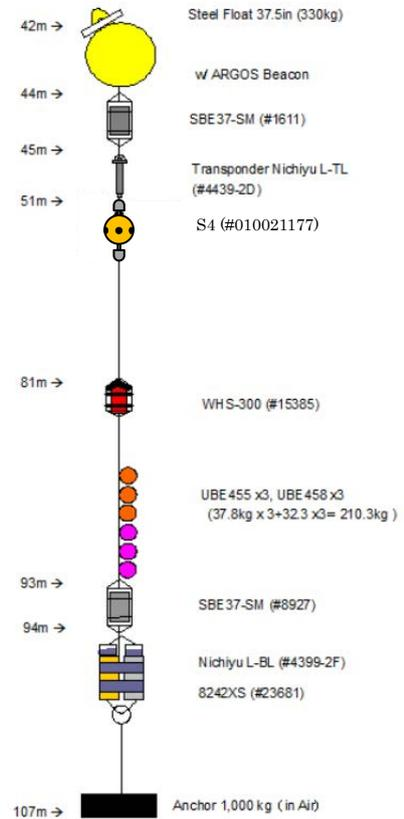
Figure 3.5-4 Mooring diagram of Deployment moorings
