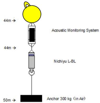
Figure 3.5-5 Mooring diagram of Deployment moorings
