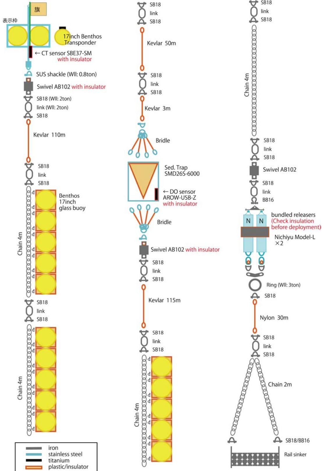
Figure 4.18-4. The layout of sediment trap mooring at Station NAP12t.
