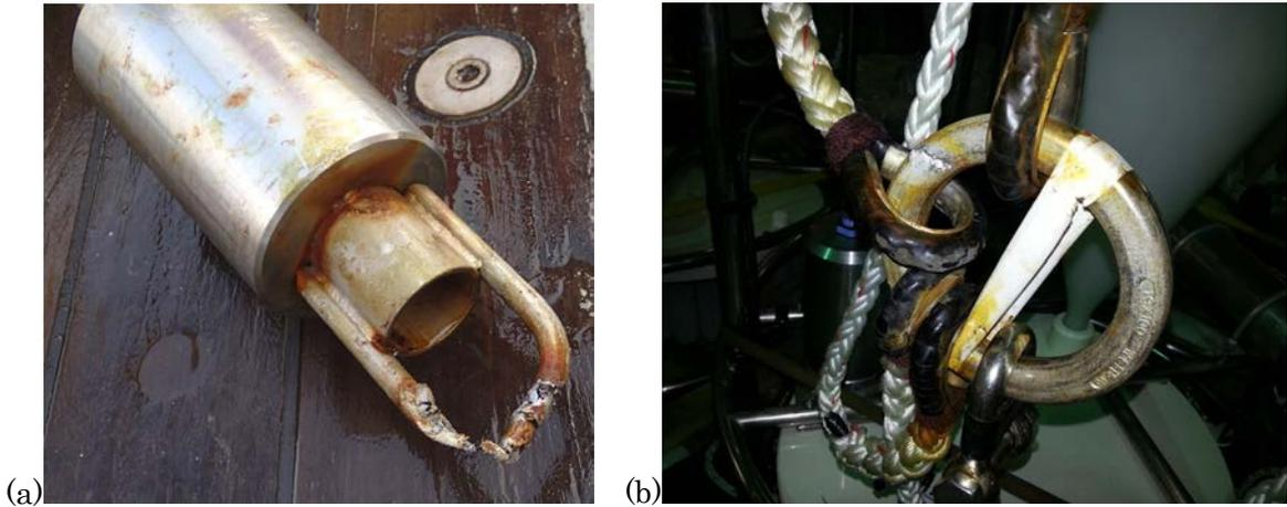
Fig. 4.18-5. The electrolytic etching of the top buoy frame and the bridal of sediment trap of NAP11t mooring. The material is stainless steel. (a) the lower end of top buoy frame; (b) the bridal ring of sediment trap.
