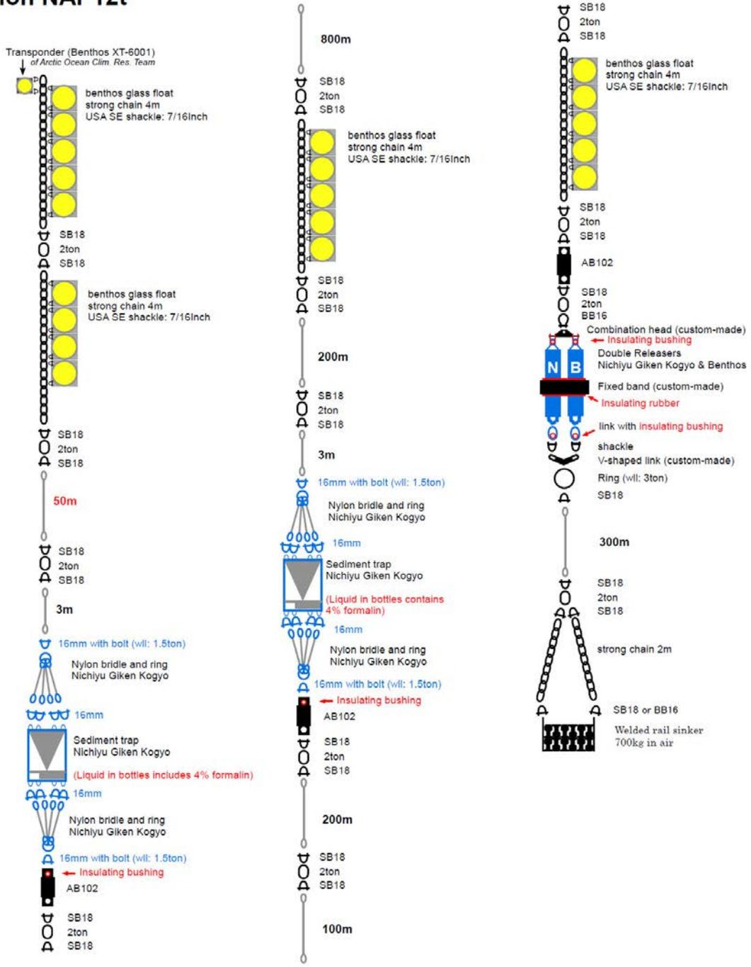
Figure 3.5-2 Mooring diagram of Deployment mooring
