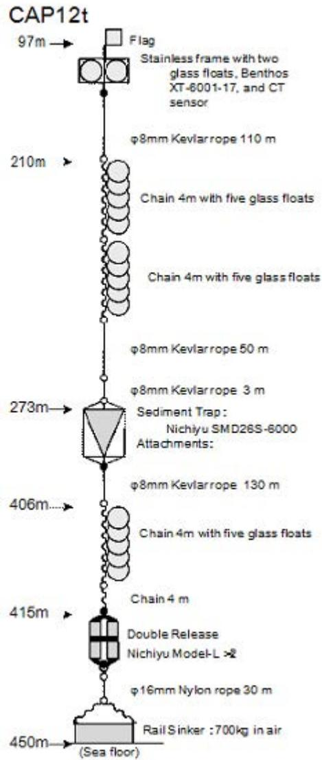
Figure 3.5-1 Mooring diagram of Deployment mooring
